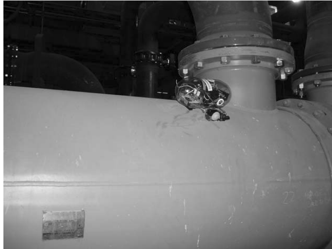
Fig. 7 MagGIE robot inspecting a pressure vessel
