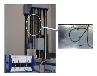
Fig. 4 Testing process of FOMDSM based on PPP-BOTDA
