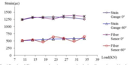
Fig. 6 Results of fiber senor and strain gauge under the bending and stretching load
