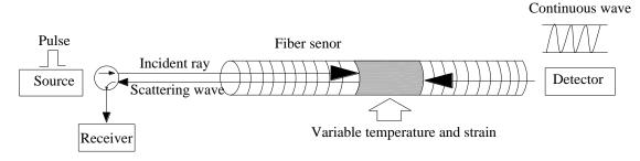
Fig. 1 Sensing principle of BOTDA
