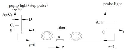
Fig. 2 Monitoring principle of PPP-BOTDA technology
