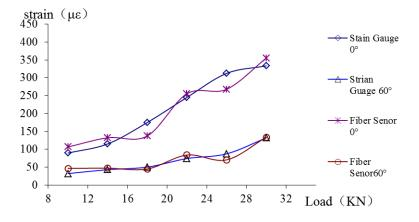
Fig. 5 Results for fiber senor and strain gauge
