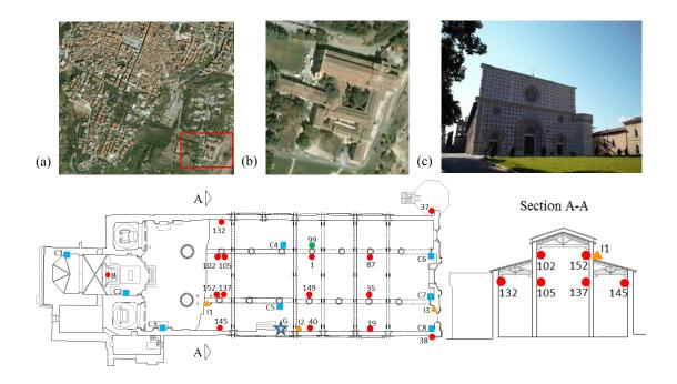
Fig. 3 On the top: Basilica of S. Maria di Collemaggio: (a) map of L'Aquila with evidence of the Basilica's location, (b) view from above, (c) main facade. On the bottom: Complete layout of the SHM system for the BSMC: 16 accelerometers (red circles, nodes 99 on the ground), 8 crackmeters (blue square), 3 inclinometers (orange triangles), 1 node gateway (star)
