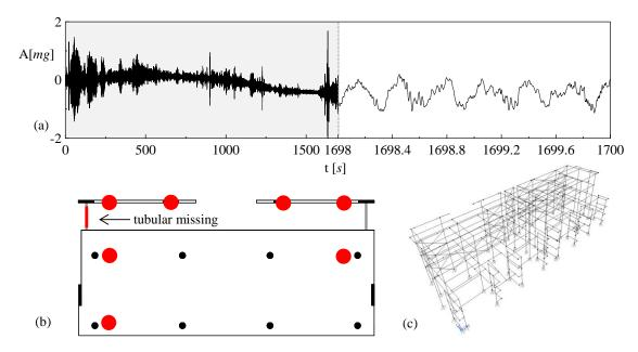
Fig. 6 (a) One of the accelerations recorded during the experimental tests, (b) Typical floor experimental layout for the substructure A3 and (c) FE model representative of the structural interaction between A3 and A4
