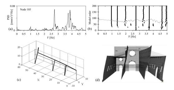
Fig. 4 Signal processing of the data acquired during the seismic events: (a) power spectral densities (PSD), (b) SSI stability diagrams, identified (c) and numerical (d) mode
