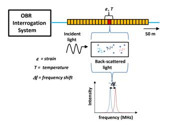
Fig. 9 Rayleigh scattering measurement process
