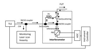
Fig. 8 Configuration of OBR setup
