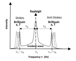
Fig. 3 Rayleigh and Brillouin spectral components in backscattered light
