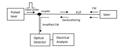
Fig. 7 Typical configuration of BOTDA setup
