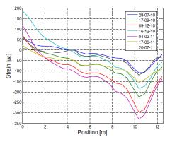
Fig. 17 Distributed compression strain measurement in the bridge
