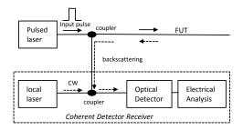
Fig. 6 Typical configuration of BOTDR setup
