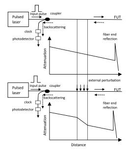
Fig. 5 Principle OTDR based on Rayleigh backscattering
