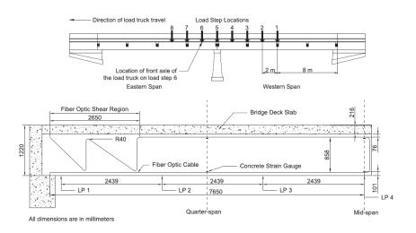
Fig. 16 Black River bridge monitoring by OBR4600 system
