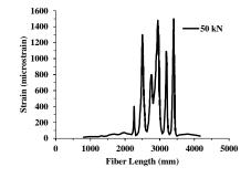
Fig. 21 Distributed strain profile performed by ODISi
