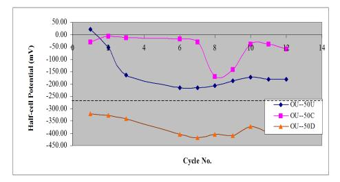
Fig. 6 Effect of epoxy coating condition on the corrosion potential of the steel reinforcing bars and its consequences on the corrosion activities
