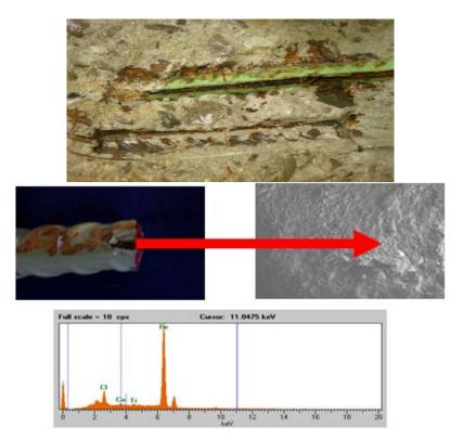
Fig. 8 The extent of corrosion occurred on epoxy coated rebar after time-to-corrosion test, confirmed by surface morphology of the steel bar under the epoxy coating layer and by the X- ray analysis that indicated the presence of chloride that instigated the corrosion process
