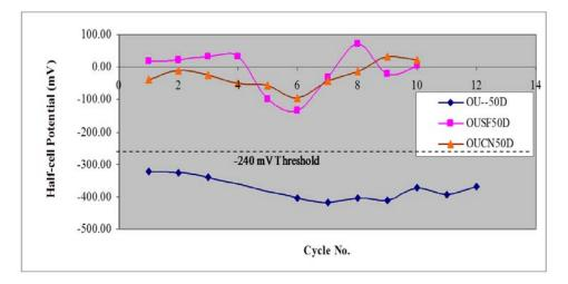
Fig. 7 Effectiveness of silica fume concrete and calcium nitrite in protecting and healing damaged epoxy coated rebars that delayed chloride ions attack on them
