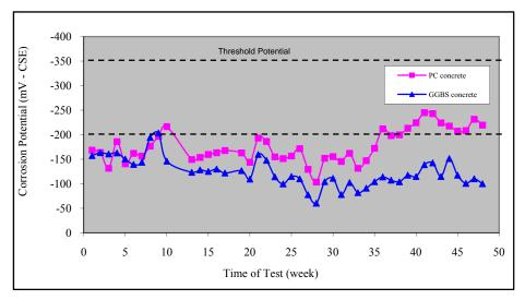
Fig. 3 Results of corrosion potential of steel reinforcing bars protected by ordinary concrete and GGBS concrete after time-to-corrosion test
