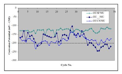
Fig. 5 Results of corrosion potential of steel reinforcing bars protected by different concretes after ASTM G-109
