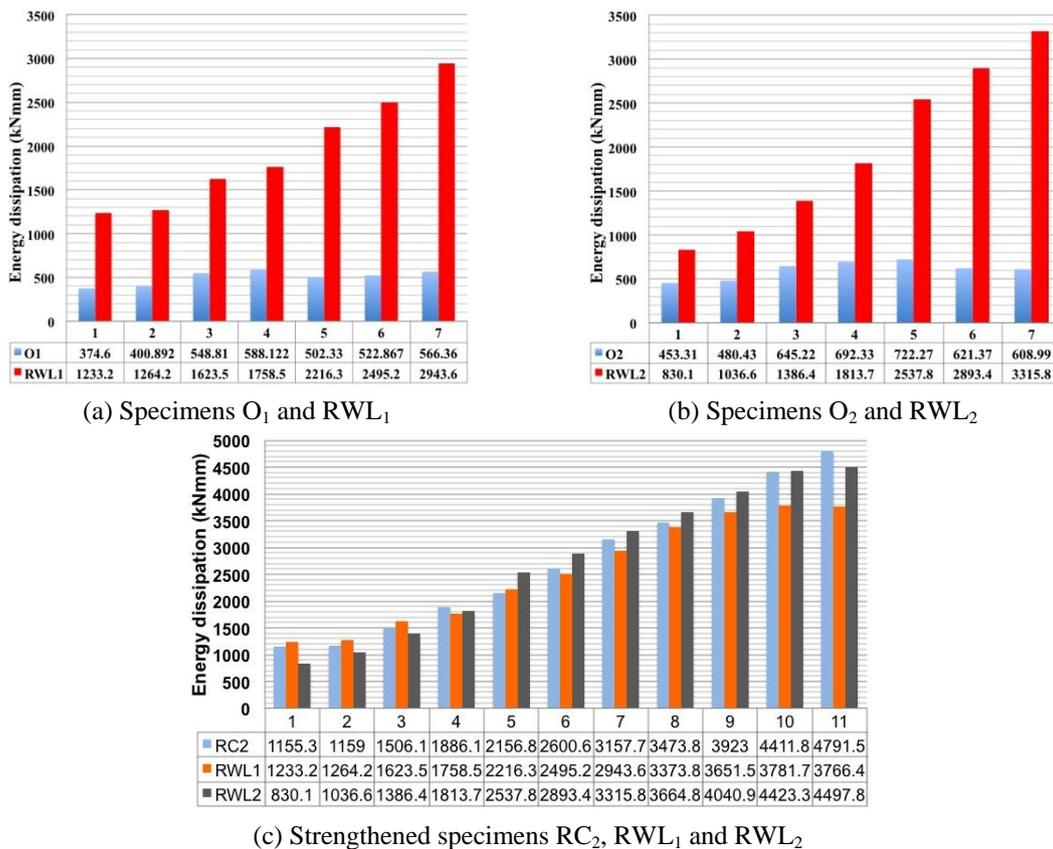
Fig. 7 Energy dissipation comparison
