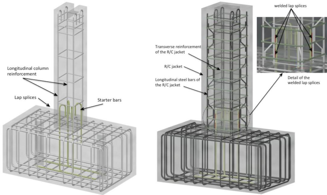
(a) Original column specimen with deficient lap splices (b) Retrofitted column via R/C jacketing and welding of the lap-spliced bars
