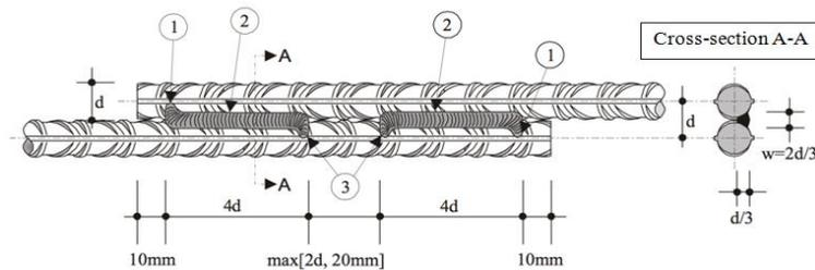
Fig. 2 Welding of the lap spliced bars according to the C.S.R.T.C (2008). 1: welding starts 10 mm from the bar end, 2: welding direction, 3: space between the welds
