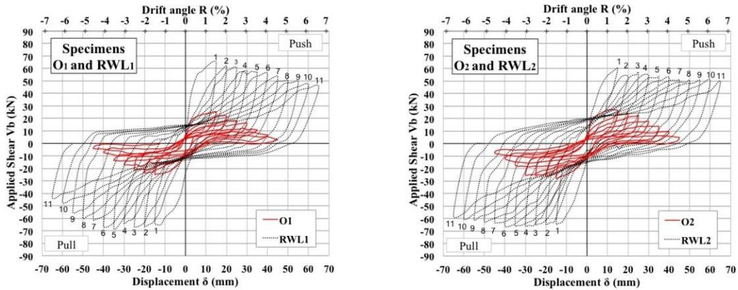
(a) Hysteretic loops of specimens  $O_1$  and  $RWL_1$  (b) Hysteretic loops of specimens  $O_2$  and  $RWL_2$
