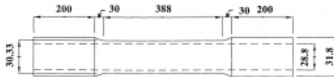
Fig. 4 Geometry of thin-walled tubular specimen (all dimensions in mm)
