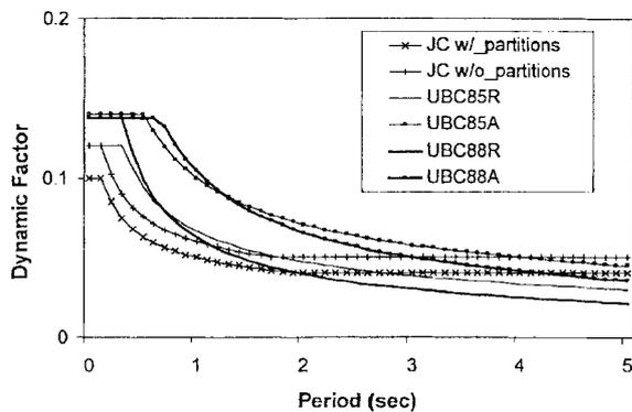
Fig. 4 Normalized dynamic factor of the JC, UBC 85 and UBC 88
