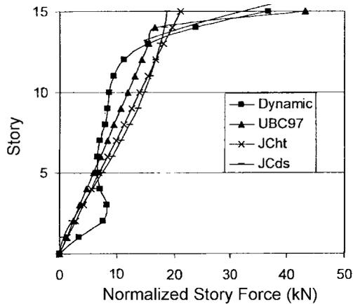
Fig. 8 Lateral load distribution for RMRF15S for JC, UBC and dynamic analysis
