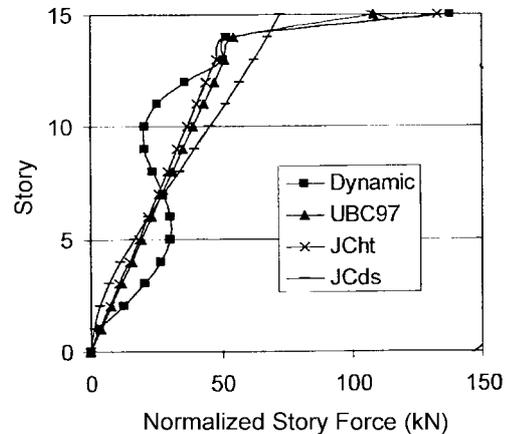
Fig. 9 Lateral load distribution for RSWF15S for JC, UBC and dynamic analysis
