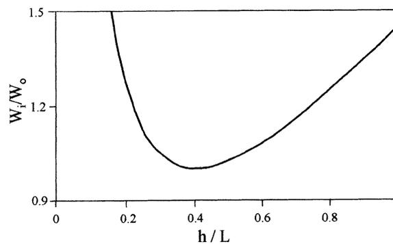
Fig. 3 Plot of arch weight versus  $h/L$  ratio for Case 1
