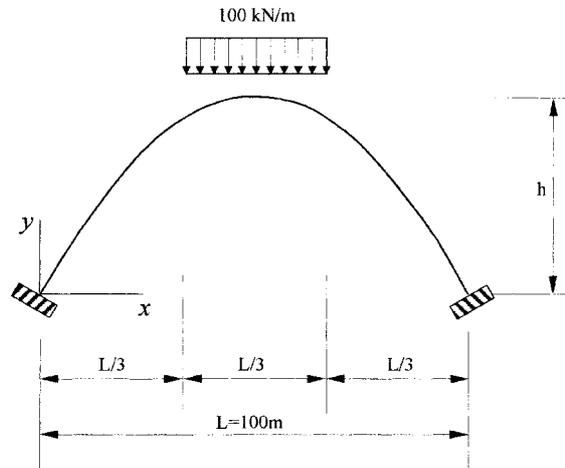
Fig. 8 A fixed arch subjected to uniformly distributed loading over the middle-third span
