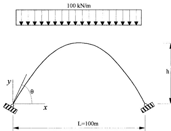
Fig. 2 A hinged arch subjected to uniformly distributed loading
