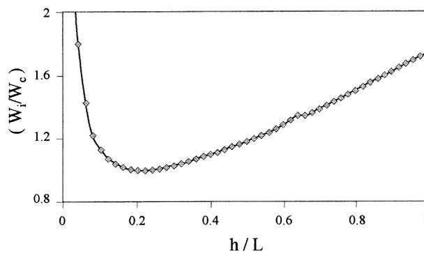
Fig. 9 Plot of arch weight versus  $h/L$  ratio for Case 3
