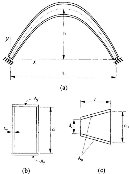
Fig. 1 A parabolic arch and its cross section
