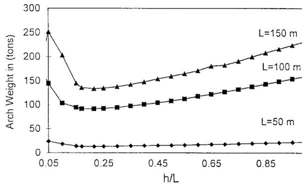
Fig. 10 Arch weight for different spans for Case 3
