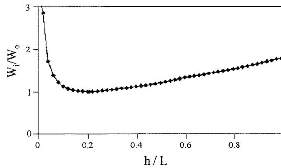
Fig. 6 Plot of arch weight versus  $h/L$  ratio for Case 2
