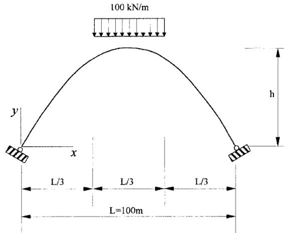
Fig. 5 A hinged arch subjected to uniformly distributed loading over the middle-third span
