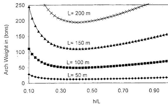
Fig. 4 Arch weight for different spans for Case 1
