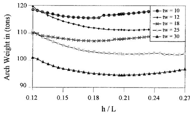
Fig. 7 Variation of arch weight for different values of  $t_w$  ( $t_w$  in mm)
