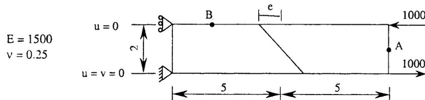
Fig. 5 Cantilever beam subjected to end bending ( $u = 0$  at the sliding node)
