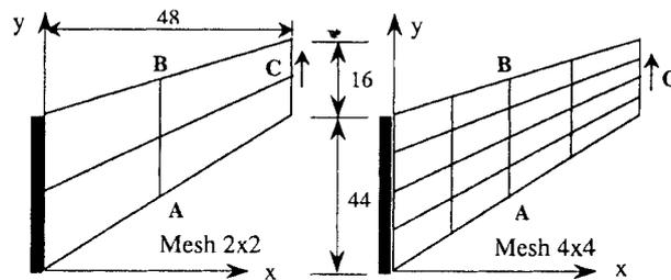
Fig. 6 Tapered panel subjected to end shear ( $E=1.0$ ,  $\nu=1/3$ )
