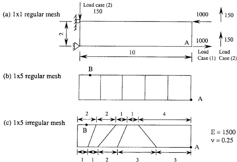
Fig. 4 Cantilever beam subjected to (1) pure bending and (2) end shear
