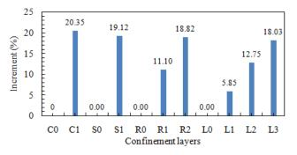
Fig. 7 Percent increment in ultimate load of various jacketed column with respect to confinement layers
