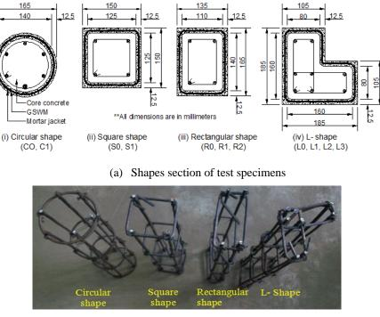
(b) Reinforcement detailing Fig. 2 Details of test specimens
