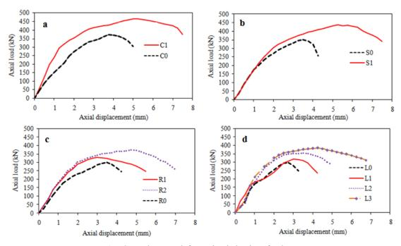
Fig. 8 Load versus deformation behavior of column
