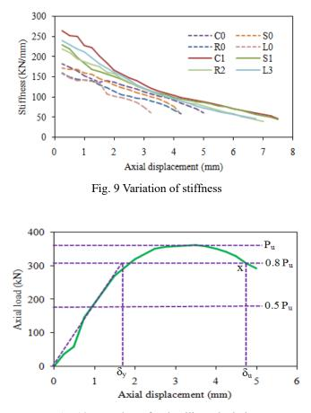
Fig. 10 Procedures for ductility calculation
