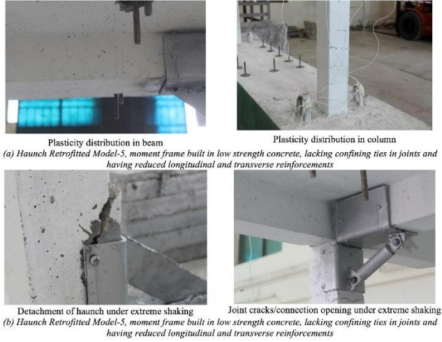
Fig. 6 Observed damages in deficient models retrofitted with Haunch
