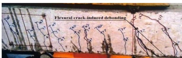
Fig. 9 Failure mode of GFRP laminated HFRC beam (HB4)
