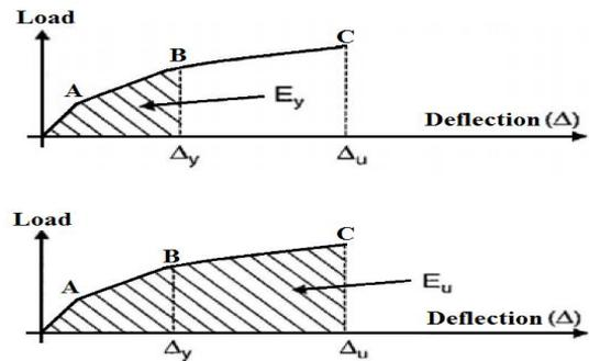
Fig. 7 Deflection ductility and energy ductility definitions
