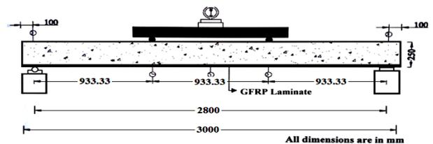
Fig. 3 Test set-up and instrumentation
