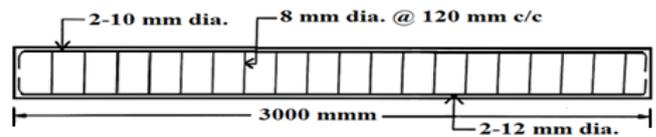
Fig. 2 Steel reinforcement details of beam
