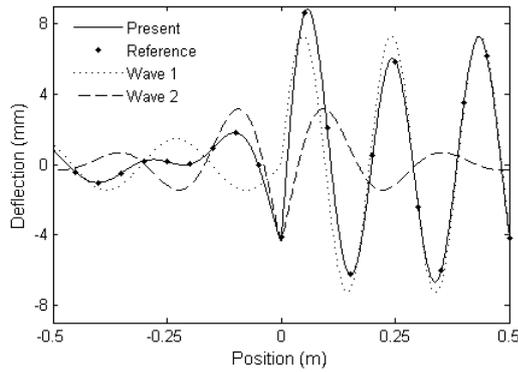
Fig. 4 Deflected shape of a Timoshenko beam on an elastic foundation subjected to a moving axle load of 2 Hz at a speed of 66.5 m/s
