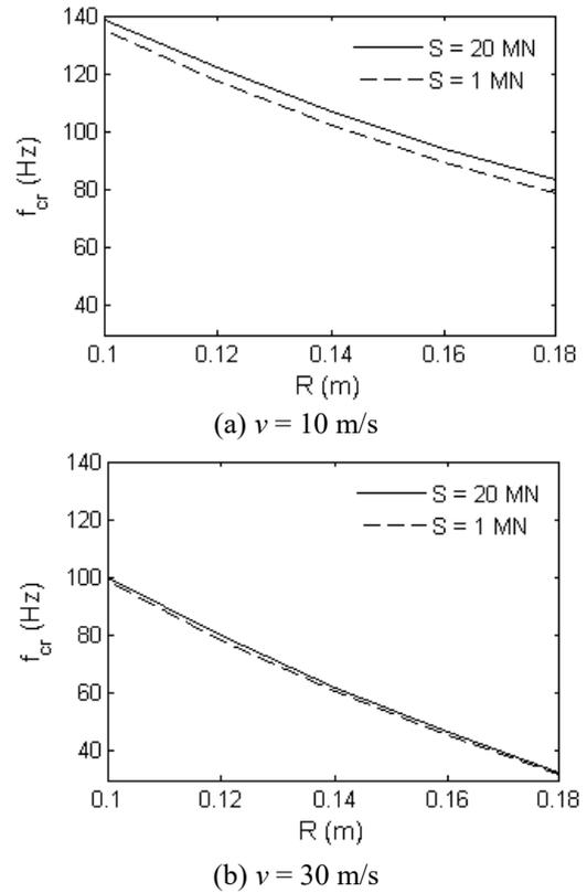
Fig. 9 Effects of the radius of gyration and the shear rigidity on the resonant frequency
