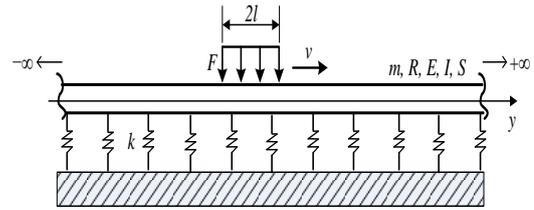
Fig. 1 An infinite Timoshenko beam on an elastic foundation
