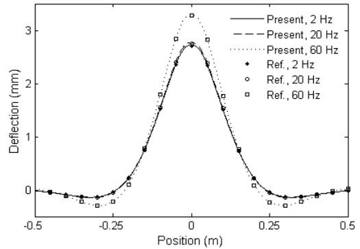
Fig. 6 Deflected shape of a Timoshenko beam on an elastic foundation subjected to a moving axle load at a speed of 30 m/s
