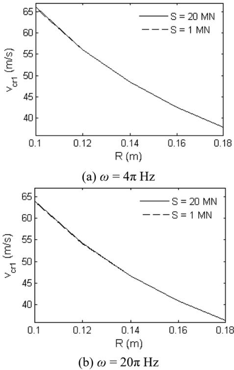
Fig. 8 Effects of the radius of gyration and the shear rigidity on the first critical velocity
