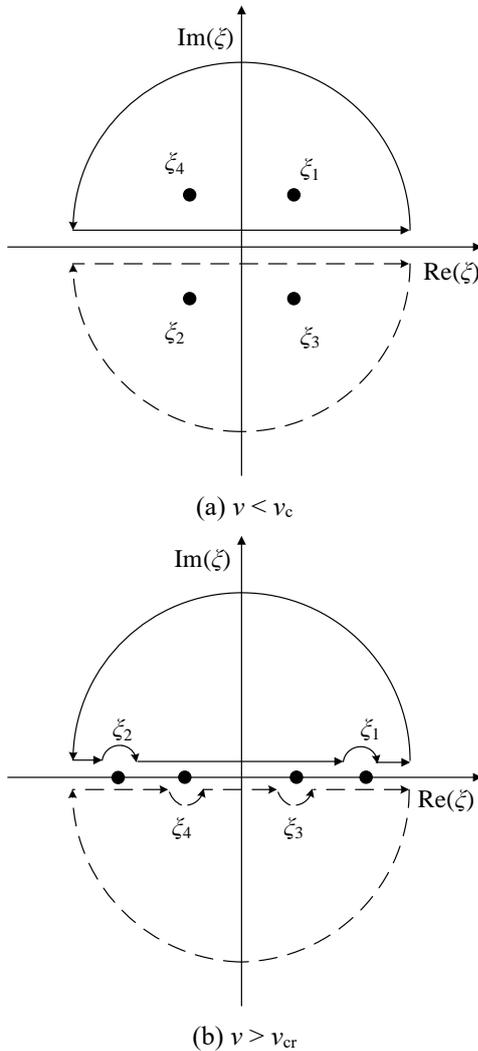
Fig. 2 Poles of the characteristic equation ( $\zeta_1$  to  $\zeta_4$ ) of an infinite EB beam on a Winkler foundation
