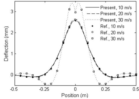
Fig. 3 Deflected shape of a Timoshenko beam on an elastic foundation subjected to a moving axle load of 2 Hz
