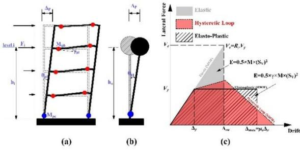
Fig. 1(a) Desired yield mechanism of special moment frame (SMF) (b) Equivalent single degree of freedom (SDOF) structure (c) Energy-work balance concept
