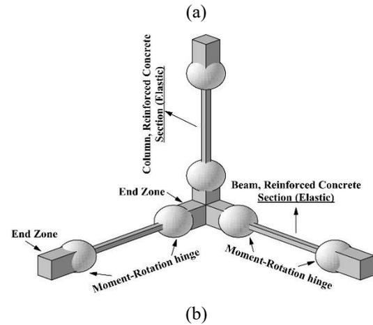
Fig. 3(a) Tri-linear curve, used to model beam-column elements (b) 3D models of beam-column elements
