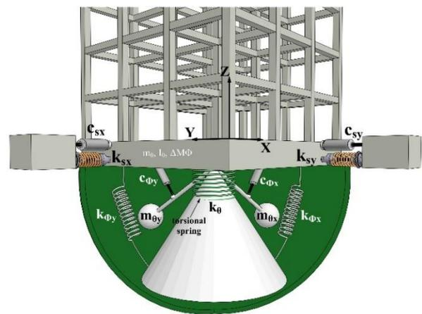
Fig. 4 Cone and spring-dashpot-mass model for foundation on surface of homogeneous half-space
