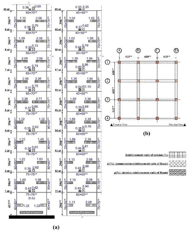
Fig. 2(a) Elevation view and (b) Plan of designed PBPD structure
