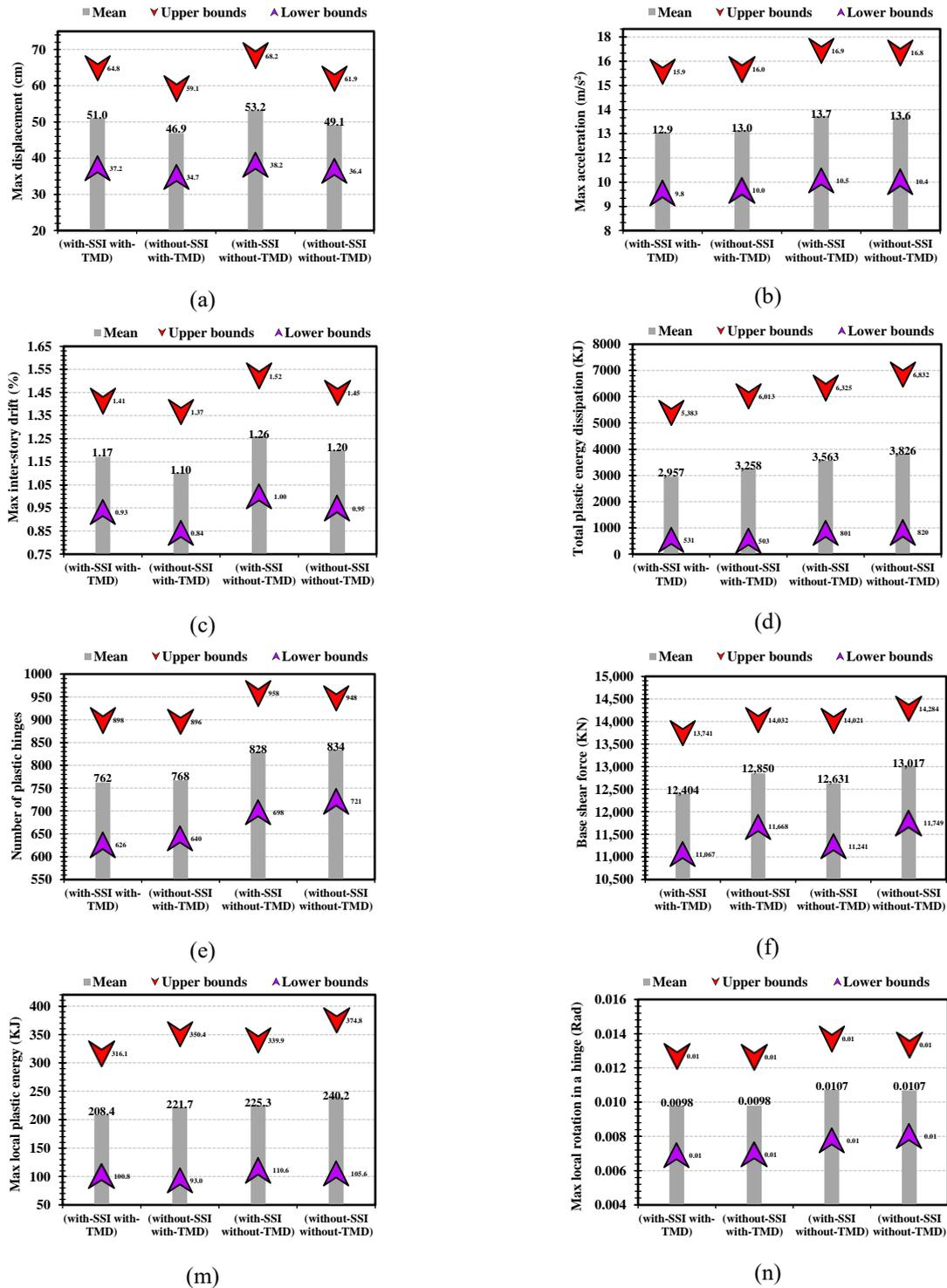
Fig. 9 Mean maximum responses and one SD of the mean of (a) displacement, (b) acceleration, (c) inter-story drift, (d) total plastic energy dissipation, (e) number of plastic hinges, (f) base shear force of structure, (m) local plastic energy and (n) local rotation in a plastic hinge in structure
