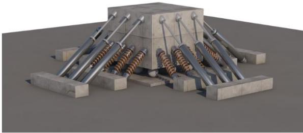
Fig. 6 TMD installed on the roof floor
