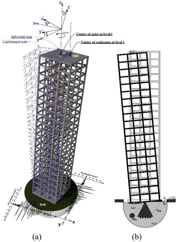
Fig. 5(a) Three-dimensional finite element models of the structure under earthquake excitations, (b) elevation of soil-structure interaction model
