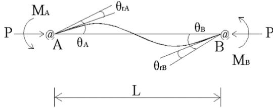
Fig. 3 Beam member with a rotational spring
