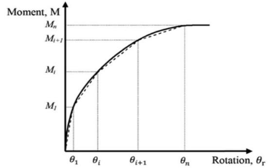
Fig. 4 Secant stiffness through the M- $\theta_r$  curve
