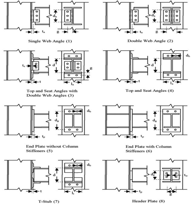
Fig. 2 Semi-rigid beam-to-column connection types (Hadidi and Rafiee 2015)
