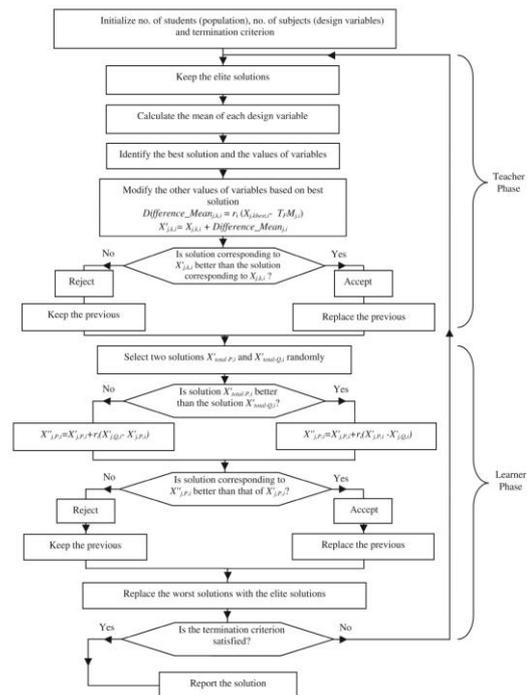
Fig. 1 Flowchart of TLBO algorithm (Rao *et al.* 2012)
