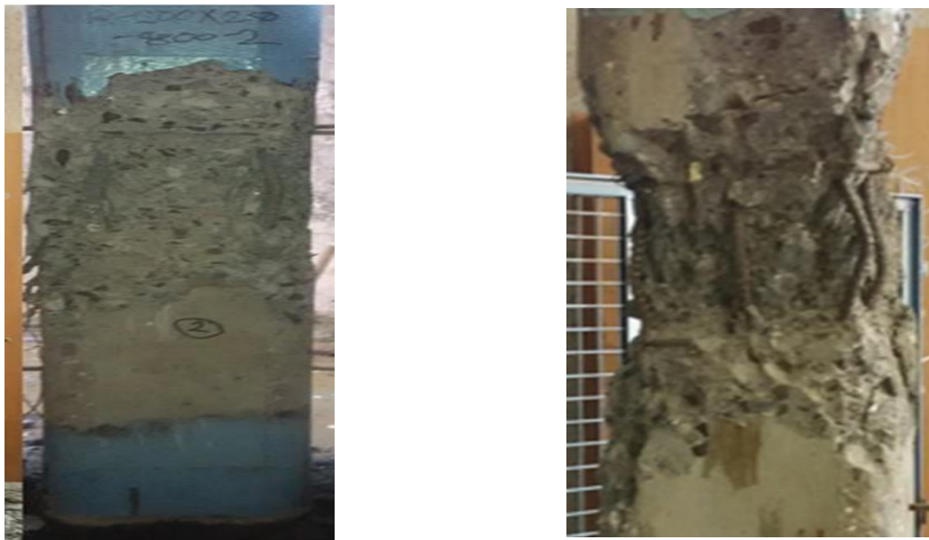
Fig. 12 Failure modes and crack patterns of unwrapped RC rectangular column
