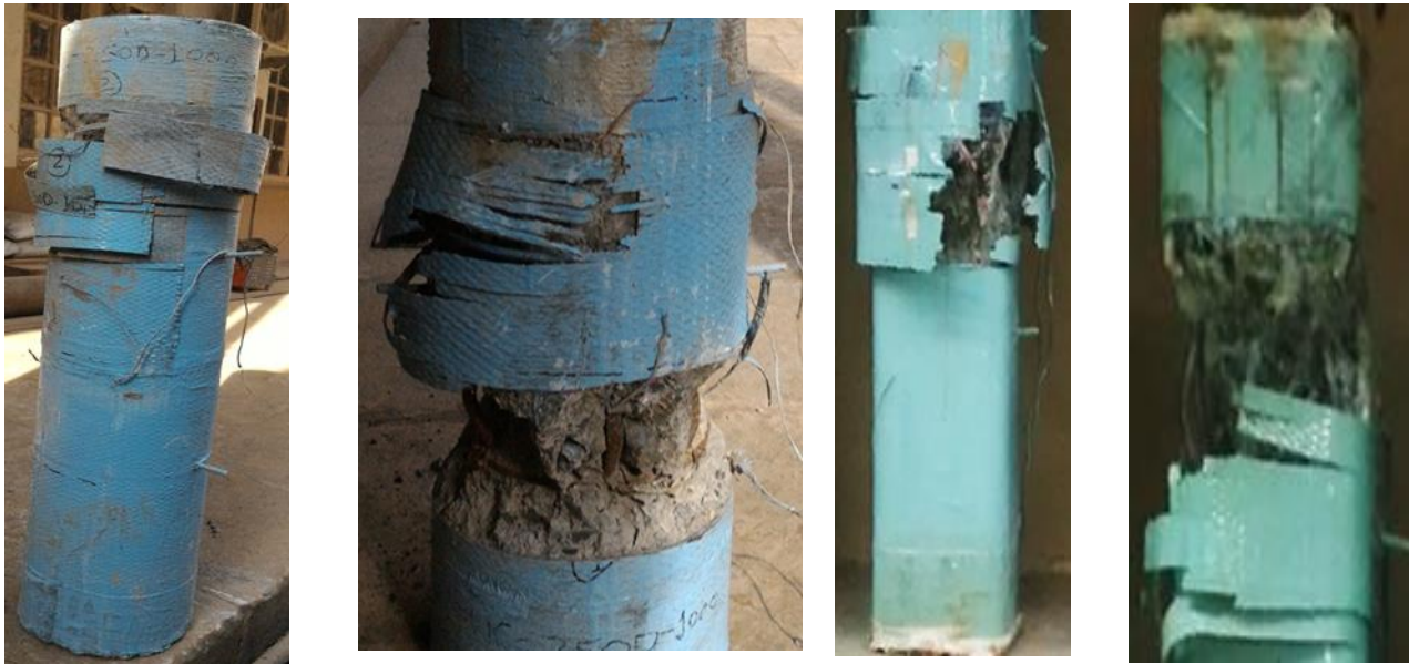
(a) Failure of CFRP wrapped circular column
