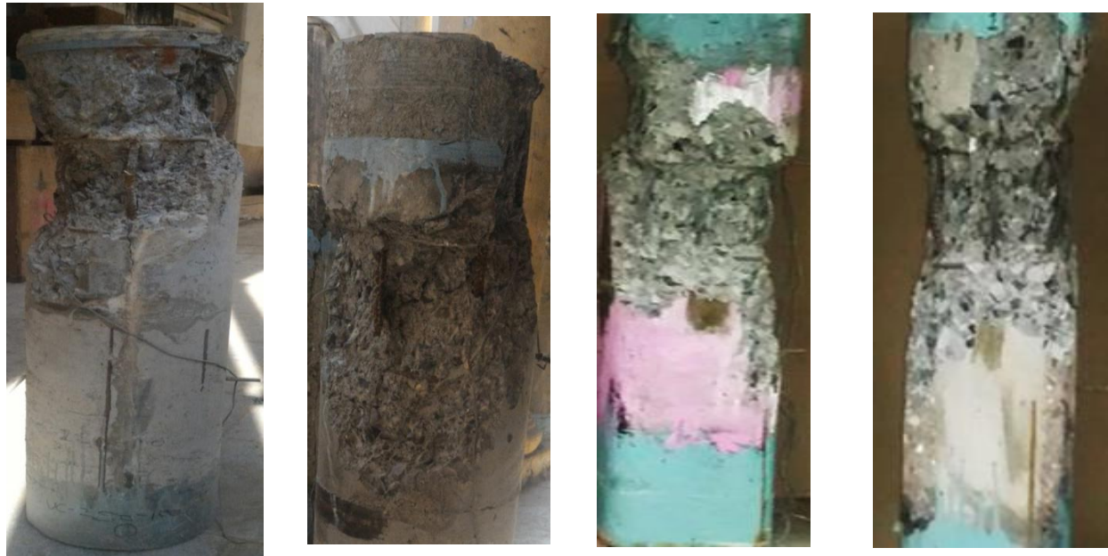
(a) Failure of unwrapped RC circular column
