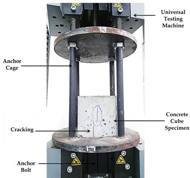
Fig. 4 Pull-out testing setup
