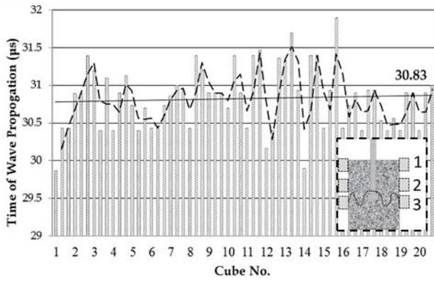
Fig. 12 Variation in ultrasonic pulse velocity along the embedment depth of anchor bolt for 12 mm  $\Phi$  anchor bolt with embedment length of 70 mm
