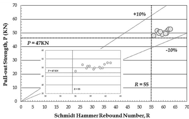
Fig. 13 Pull-out load versus rebound number relationship for 12 mm  $\Phi$  anchor bolt with embedment length of 70 mm
