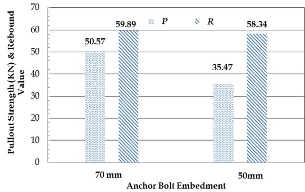
Fig. 14 Average pull-out load versus rebound number comparison for 12 mm  $\Phi$  anchor bolt
