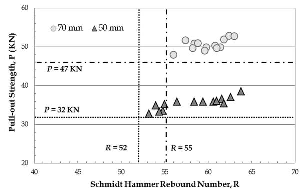
Fig. 15 Combined pull-out load carrying capacity versus Schmidt hammer rebound number
