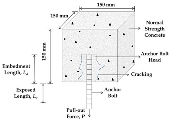
Fig. 7 Schematic diagram showing anchor bolt installation and cracking pattern
