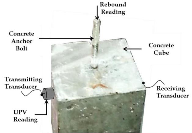
Fig. 3 Cube specimen depicting the Schmidt hammer and UPV testing
