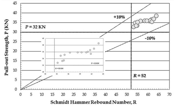
Fig. 11 Pull-out load versus rebound number relationship for 12 mm  $\Phi$  anchor bolt with embedment length of 50 mm
