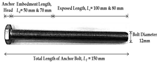
Fig. 1 Sample anchor bolt
