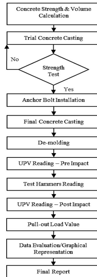
Fig. 5 Flow chart of research methodology and effective test setup
