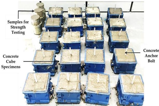
Fig. 2 Concrete samples for testing
