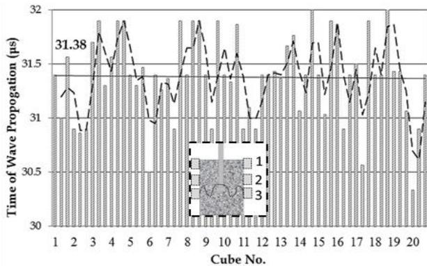
Fig. 10 Variation in ultrasonic pulse velocity along the embedment depth of anchor bolt for 12 mm  $\Phi$  anchor bolt with embedment length of 50 mm
