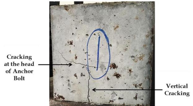
Fig. 8 Crack along the anchor bolt embedment length
