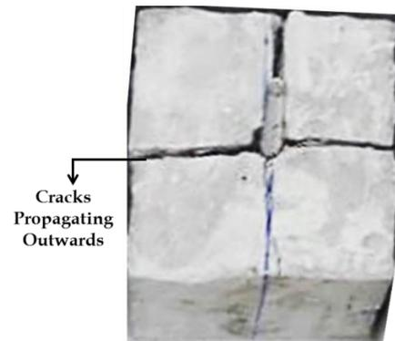
Fig. 9 Cracking on top of the anchor bolt
