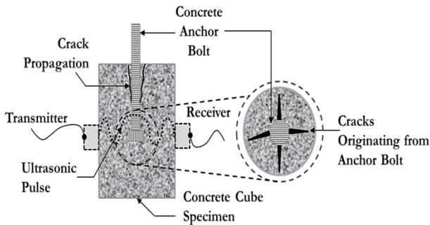
Fig. 6 Conceptual diagram of crack propagation around the embedded anchor bolt
