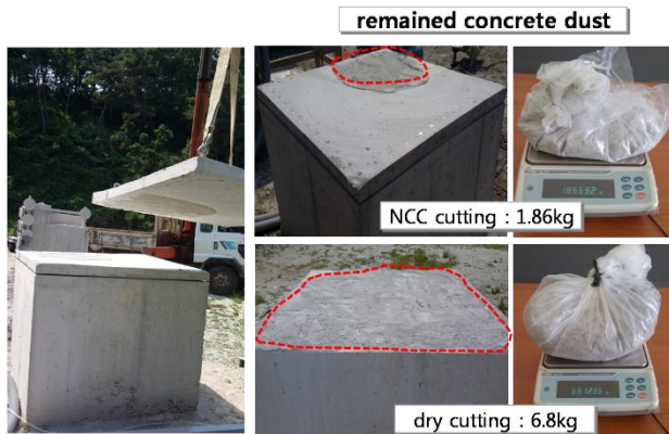
Fig. 24 Remaining dust comparison between NCC method and dry cutting method
