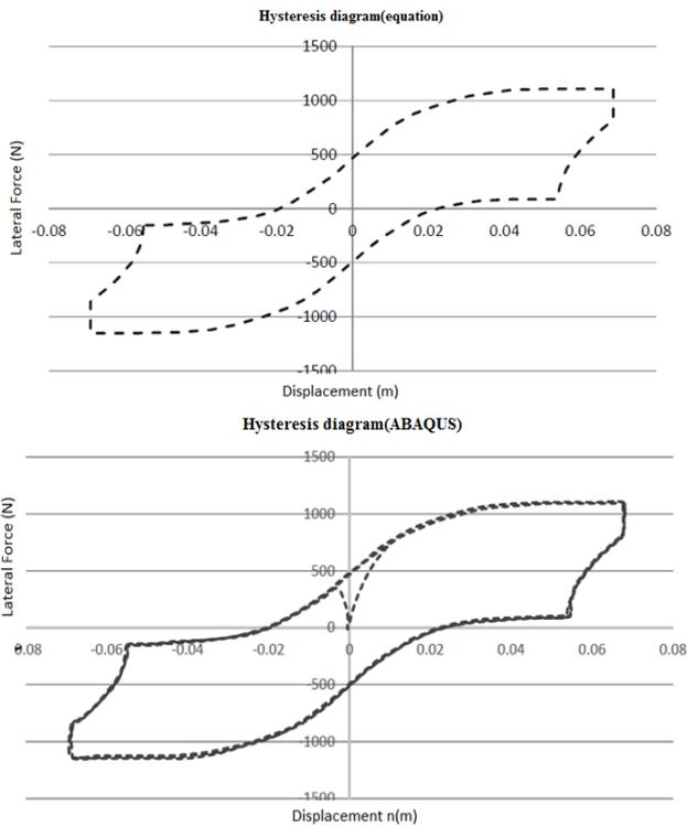
Fig. 7 Hysteresis diagram of DVFPI isolator, in the 4th case (unequal geometry equal friction)
