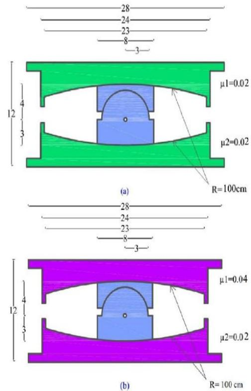
Fig. 1 Sample DCFP isolators modeled (a) with equal friction, and (b) with unequal friction
