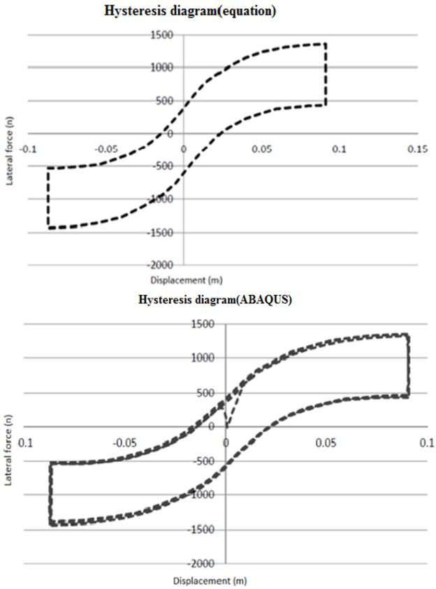
Fig. 4 Hysteresis diagram of DVFPI isolator with equal geometry and friction
