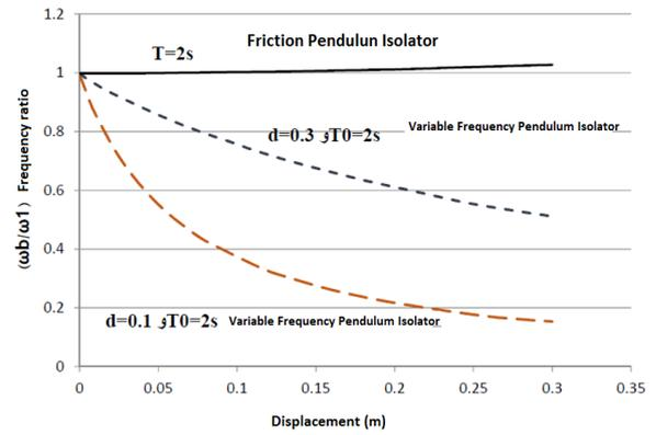
Fig. 8 Effect of parameter  $d$  on the decrease of frequency with respect to displacement compared to DCFP isolator (Mashaieghi 2015)
