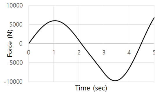
Fig. 18 Exciting force applied to each one of the loaded nodes
