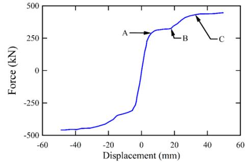
Fig. 7 The experimental pushover curve of the CK-VLB1
