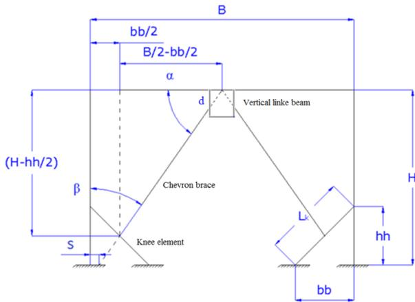
Fig. 3 Geometrical characteristics of the structure
