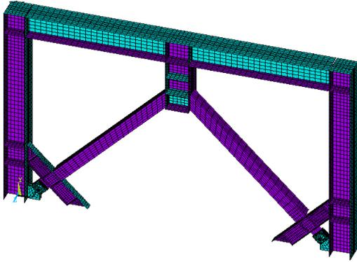
Fig. 12 Finite element model of the proposed two-level control system
