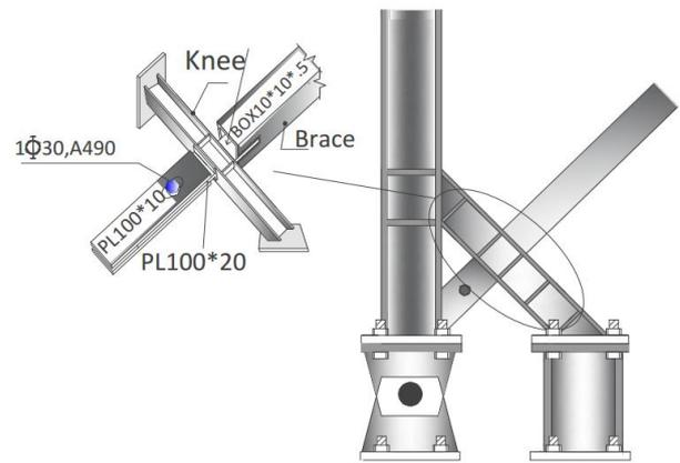
Fig. 4 Schematic of stopping system and slotted bolted connection
