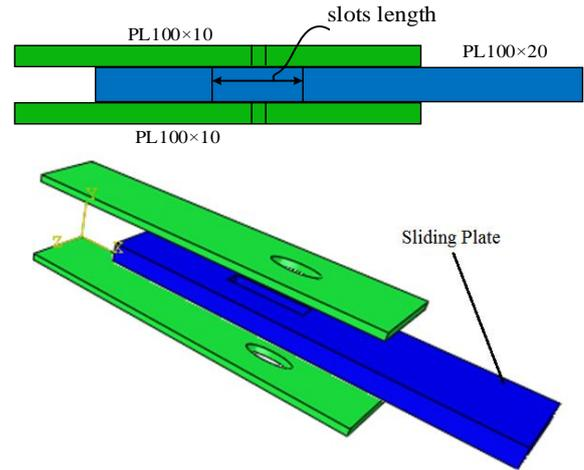
Fig. 2 Proposed slotted bolted stopper details
