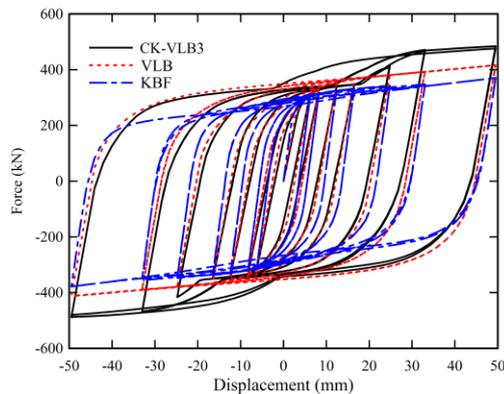
Fig. 16 Comparison between the proposed CK-VLB3 sample model hysteresis curve, KBF and VLB bracing systems
