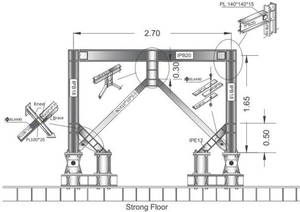
Fig. 1 General geometry of the proposed two-level control system along with its connection details
