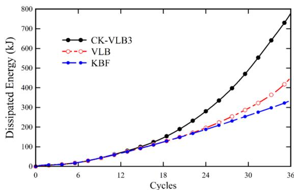
Fig. 17 Comparison of the cumulative dissipated energies of CK-VLB3 with those of vertical link and knee bracing systems
