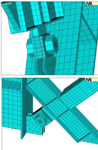
Fig. 13 Detailed meshing for presented stopping mechanism
