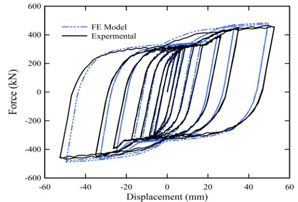
Fig. 14 Hysteresis loop of calibrated numerical model and test results for CK-VLB3
