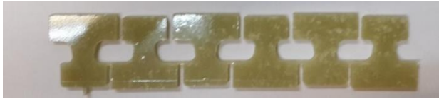
Fig. 1 CSM/epoxy composite specimens based on B593-96 ASTM Standard (2003)
