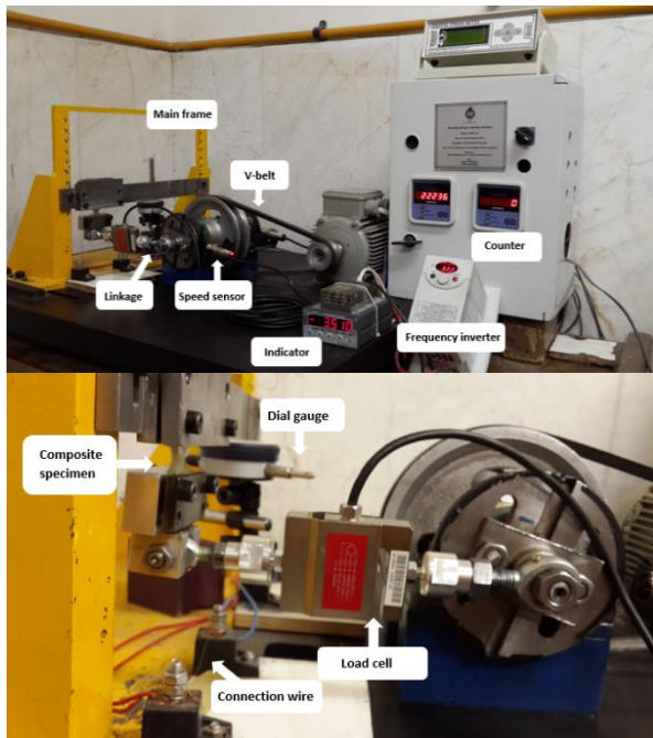
Fig. 2 The experimental setup for the displacement-controlled flexural fatigue loading (BFM-110)
