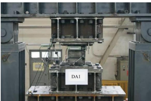
Fig. 3 Test setup on steel damper
