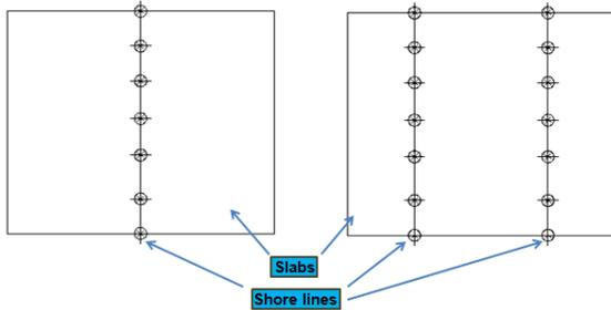
Fig. 3 Plan view of a slab with (a) a single line of shores and (b) double line of shores
