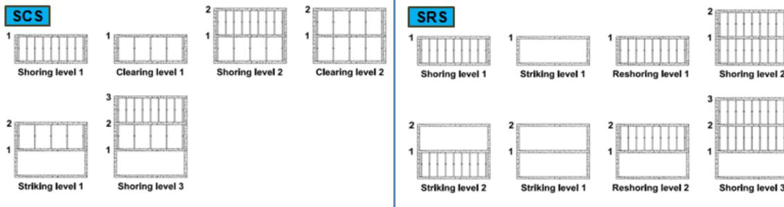
Fig. 2 Construction phases up to the shoring of Level 3 for SCS and SRS of a building with 2 consecutively shored floors
