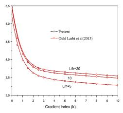
Fig. 5 Variation of the non-dimensional fundamental frequency  $\overline{w}$  of an FG beam with the gradient index *k* and span-to-depth ratio L/h
