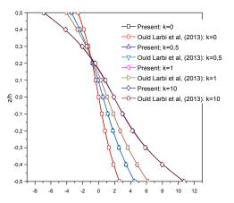
Fig. 1 The variation of the axial displacement  $\overline{u}$  through the thickness of an FG beam (*L*=2*h*)
