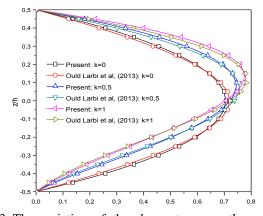
Fig. 3 The variation of the shear stress  $\bar{\tau}_{xz}$  through the thickness of an FG beam (*L*=2*h*)
