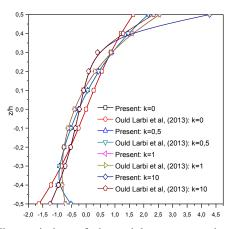
Fig. 2 The variation of the axial stress  $\overline{\sigma}_x$  through the thickness of an FG beam (*L*=2*h*)
