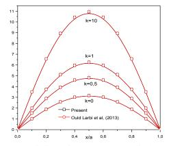
Fig. 4 The variation of the transverse displacement  $\overline{w}$  versus non-dimensional length of an FG beam (*L*=5*h*)
