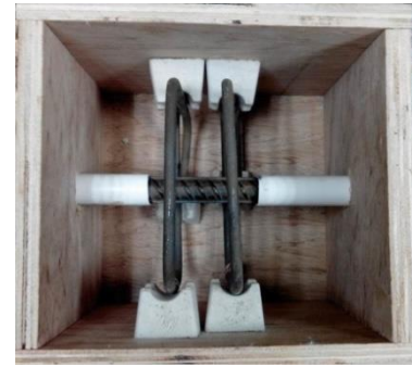
Fig. 2 Mould and reinforcement
