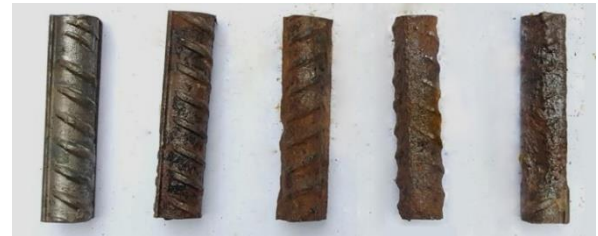
Fig. 5 Rebars at different corrosion levels from left to right: 0.13%, 3.45%, 6.87%, 9.55%, 14.60%
