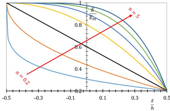
Fig. 2 Distribution of dimensionless modulus of elasticity versus  $z/h$  at  $x=0$
