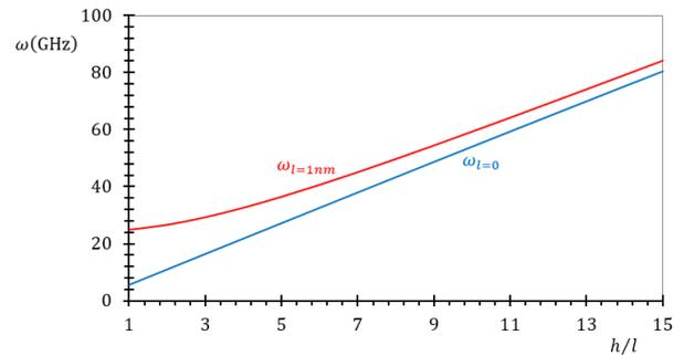
Fig. 6 Frequency of clamped-clamped BDFG nano beam by considering the effects of couple-stress theory and the classic theory versus to dimensionless thickness ( $L=100$  nm,  $b=h$ ,  $n=2$ ,  $\beta=2$ , and  $l=1$  nm)
