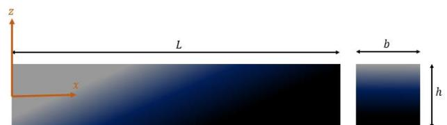
Fig. 1 Geometry of the bi-directional functionally graded Euler-Bernoulli nano-beam
