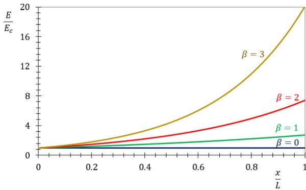
Fig. 3 Distribution of dimensionless modulus of elasticity versus  $x/L$  at  $z=h/2$
