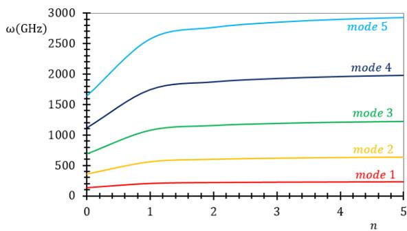
Fig. 8 Frequency of clamped-clamped BDFG nano-beam versus  $n_1=n_2=n$  in different modes ( $b=h=5$  nm,  $L=75$  nm,  $\beta=2$ , and  $l=5$  nm)
