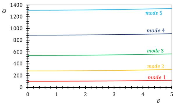
Fig. 9 Dimensionless frequency of clamped-clamped FG nano-beam versus  $\beta$  in different modes ( $b=h=5$  nm,  $L=75$  nm,  $\beta=2$ , and  $l=5$  nm)
