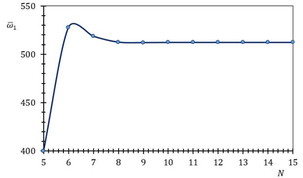
Fig. 4 Convergence of dimensionless frequency in mode 1 clamped-clamped BDFG ( $\beta=2$ ,  $n=2$ ,  $b=h=1$  nm,  $L=100$  nm, and  $l=5$  nm)
