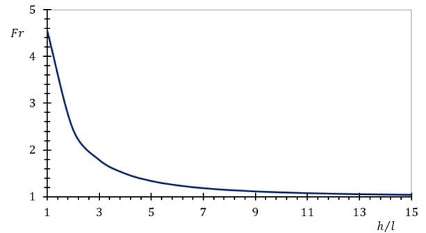
Fig. 5 Frequency ratio of clamped-clamped BDFG nano beam versus to dimensionless thickness ( $L=100$  nm,  $b=h$ ,  $n=2$ ,  $\beta=2$ , and  $l=1$  nm)
