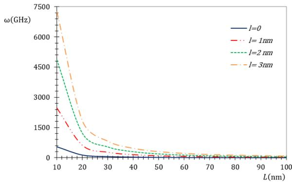
Fig. 7 Frequency in mode 1 of clamped-clamped BDFG nano beam versus to length in various values of  $l$  ( $b=h=1$  nm,  $n=2$ ,  $\beta=2$ , and  $l=5$  nm)
