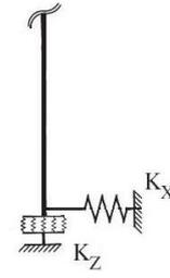
Fig. 4 Multi-spring model for the SDOF foundation support
