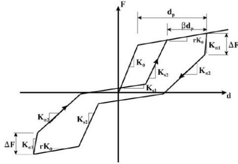
Fig. 3 Pampanin pinching and stiffness degrading hysteresis loop (Carr 2008)
