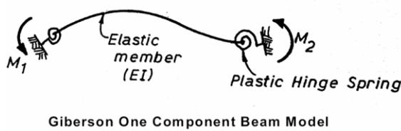
Fig. 8 Lumped plasticity beam-column element (Arefi 2008)
