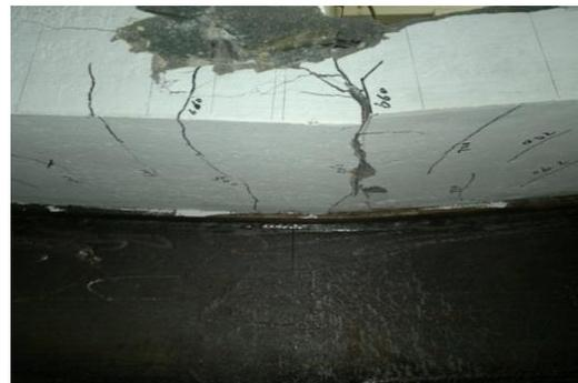
Fig. 9 Cracks of bending failure
