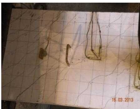
Fig. 7 Cracks on top of beam
