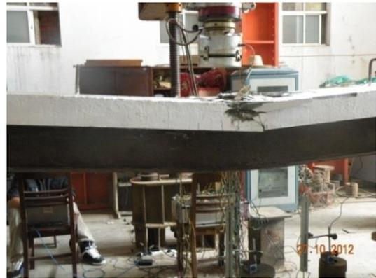
Fig. 8 Bending failure of beam
