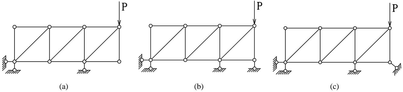
Fig. 1 The truss structures. (a) initial design, (b) modified design with added one support along vertical axis of the global coordinate system, (c) modified design with added one skew support
