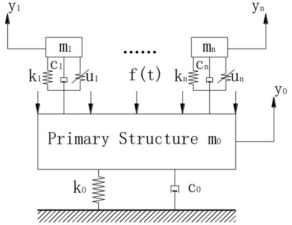
Fig. 2 Computational model of pedestrian bridge system with MTMD
