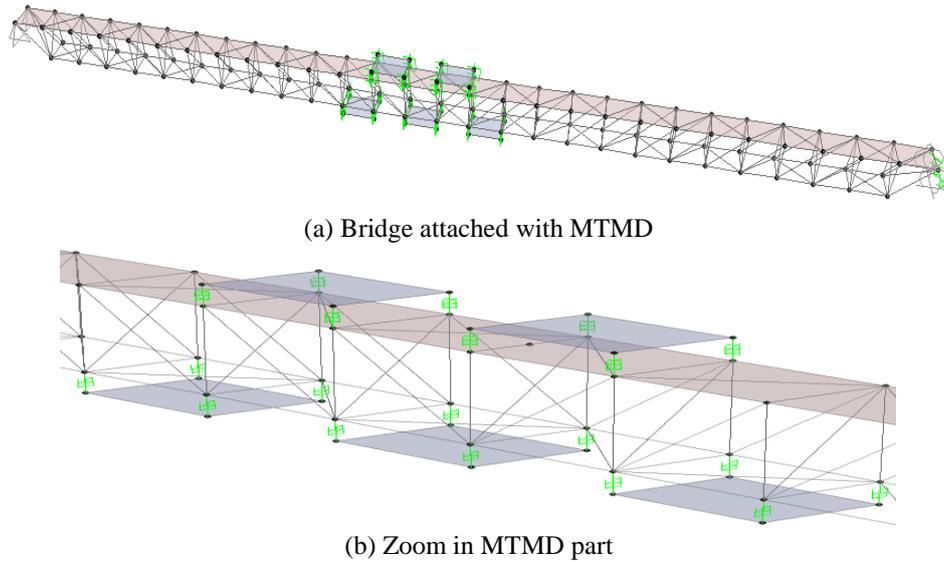
Fig. 4 Model of bridge in SAP2000
