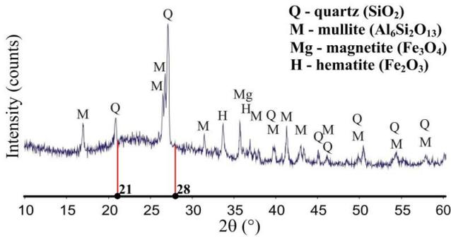
Fig. 2 XRD pattern of the Fly ash
