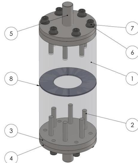
Fig. 4 The Device for fracture toughness test in the Mode III fracture: 1-concrete specimen, 2-bolt M12/65, 3-bottom plate, 4-top plate, 5-bolt M28/70, 6-washers, 7-bolt M12/20, 8-insert
