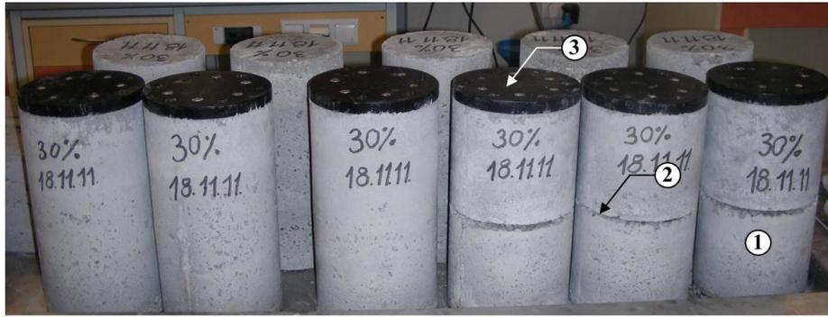
Fig. 5 A group of devices prepared to fracture toughness tests: 1-concrete specimen, 2-initial crack 3-concreted bottom plate
