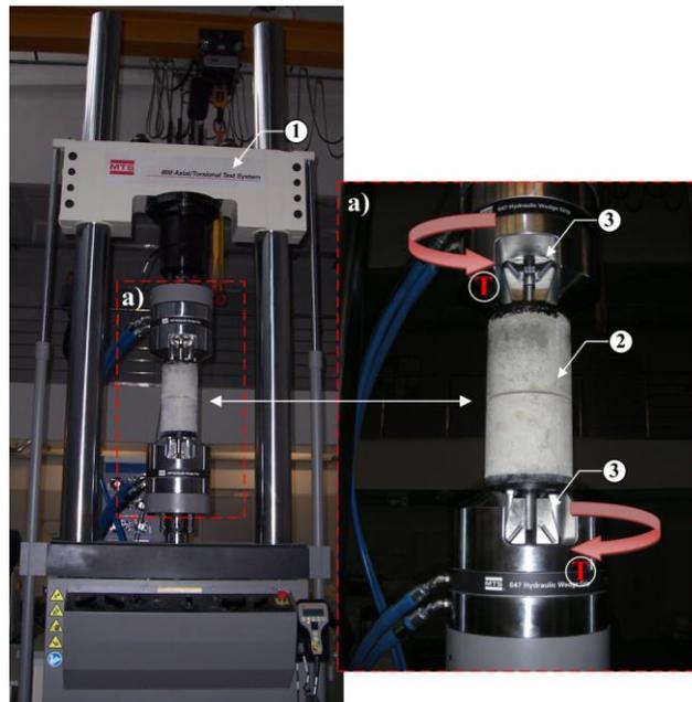
Fig. 6 The experimental stand with the fixed specimen subjected to torsion: a) a detail of the mounting device for testing of the fracture toughness; 1-MTS 809 press, 2-device for testing of the fracture toughness, 3-the grips of the press,  $T$ -torque
