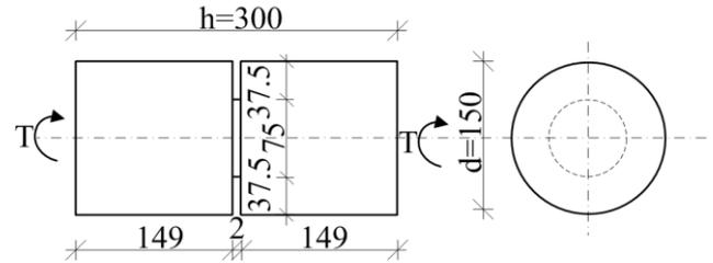
Fig. 3 Geometrical configuration of tested specimen (dimensions in mm), *T*-torque
