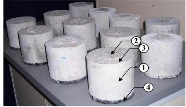
Fig. 8 A view of fractured specimens after the fracture toughness test, showing the failure surfaces; 1-a half of the cylinder, 2-failure surface, 3-the place where the insert was placed, 4-bottom plate
