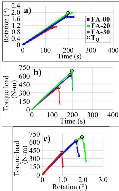
Fig. 7 Examples of graphs obtained from the testing: (a)  $\theta$  vs  $t$ , (b)  $T$  vs  $t$ , (c)  $T$  vs  $\theta$
