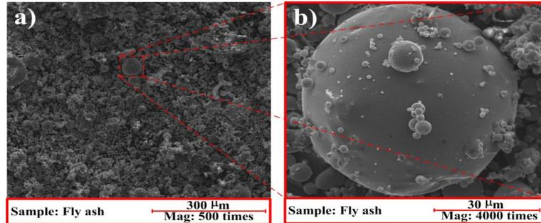
Fig. 1 Microstructures and grains of used FA: (a) grains (Magnification: 500 times), (b) grain with cenospheres (Magnification: 4000 times)
