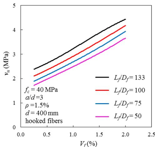
Fig. 8 Shear strength vs. volume fraction of fibers
