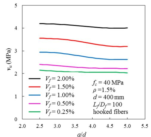
Fig. 13 Shear strength vs. shear span-to-depth ratio
