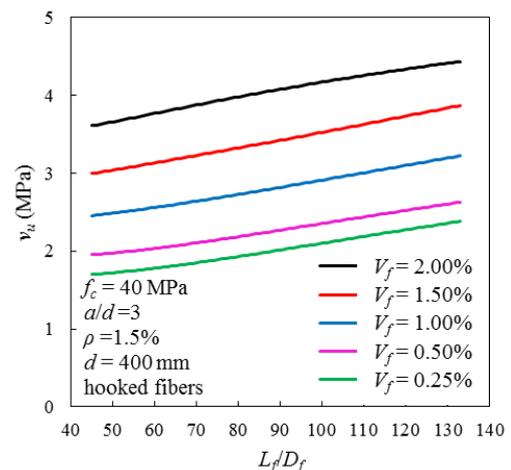
Fig. 9 Shear strength vs. aspect ratio of fibers
