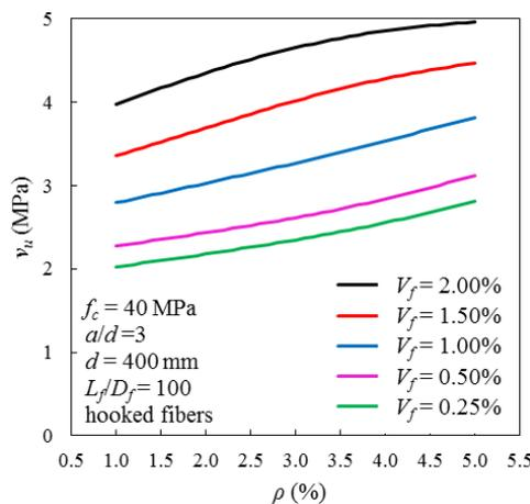
Fig. 12 Shear strength vs. tensile reinforcement ratio
