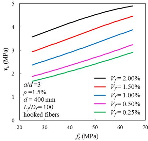
Fig. 10 Shear strength vs. concrete compressive strength
