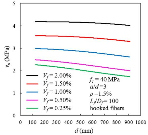
Fig. 11 Shear strength vs. effective depth
