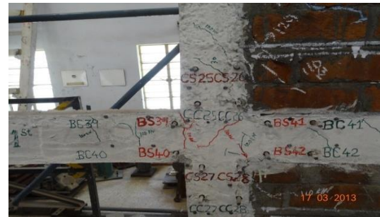
Fig. 9 Map cracks in the column-beam junction of normal frame
