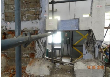
Fig. 12 Shear buckled cracks in the leeward column of retrofitted frame
