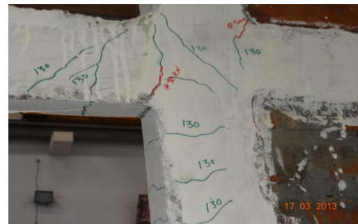
Fig. 10 Cracks at the tension zones
