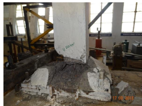
Fig. 11 Hinge formation at leeward column of normal frame
