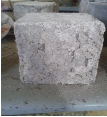
Fig. 8 Specimen after subjected to curing in acid
