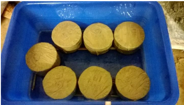
Fig. 12 Specimens being tested for water absorption
