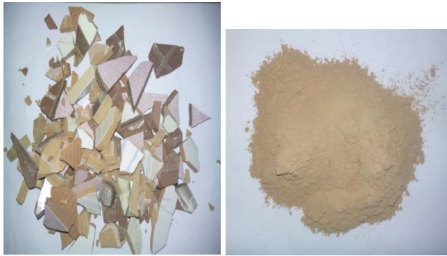
Fig. 2 Ceramic before and after grinding in Ball Mill
