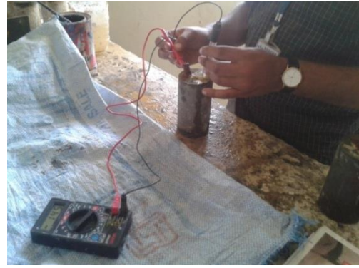
Fig. 9 HCP tests being performed on specimens
