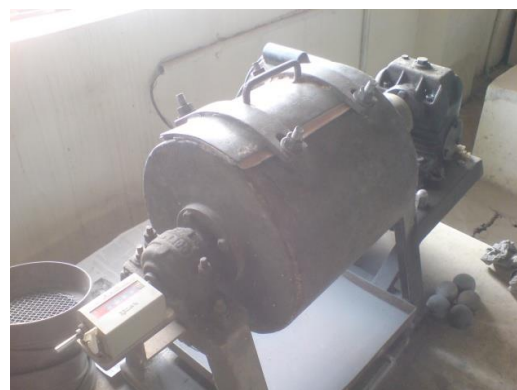
Fig. 1 Ball mill used for grinding ceramic tiles
