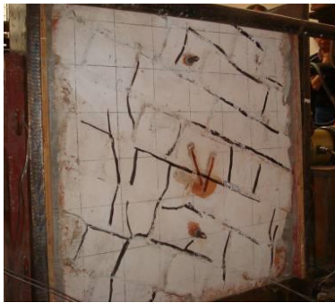
(a) Mortar extruded and cracks appeared
