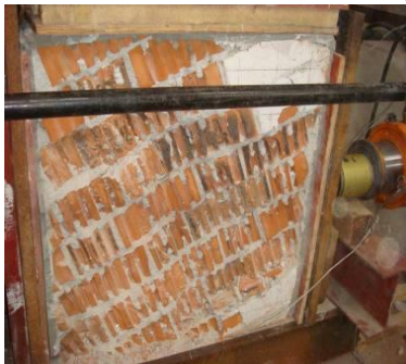
(e) Bricks' face shell flaked off (small number of panels)
