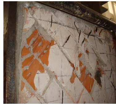
(b) Cracks expanding and deformation out of plane
