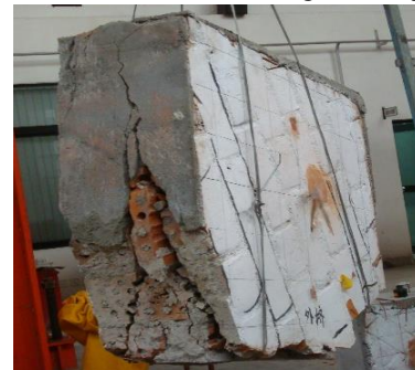
(f) Spalling with crushing damage at mid-thickness
