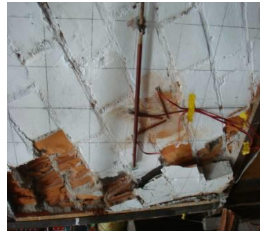
(d) Failure occurred at the edge of the panel
