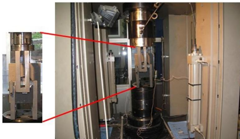
Fig. 8 Compression load frame
