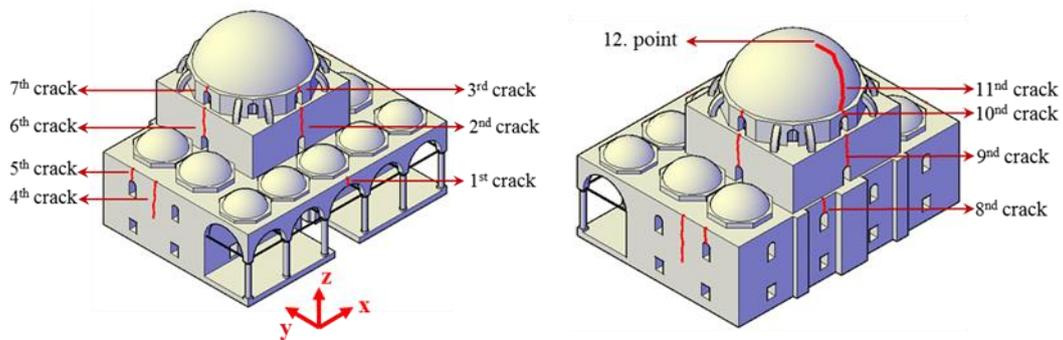
Fig. 2 Existing cracks on Hafsa Sultan mosque
