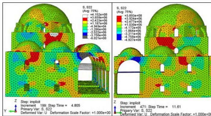
Fig. 8 Stress concentrations on model calibrated of Hafsa Sultan mosque ( $\sigma_{22}$ )
