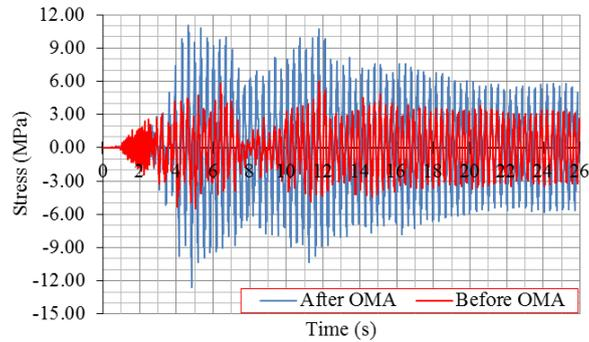
Fig. 7 The stresses in the direction  $x$  in the first crack zone ( $\sigma_{11}$ )
