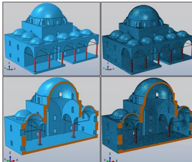
Fig. 3 Three-dimensional finite element model of Hafsa Sultan mosque
