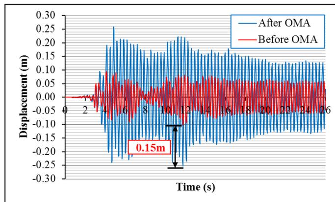
Fig. 6 Comparison of maximum displacement time graph in the main dome peak point
