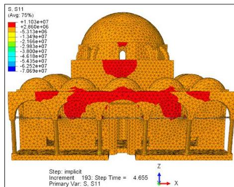
Fig. 9 Stress concentrations on model calibrated of Hafsa Sultan mosque ( $\sigma_{11}$ )
