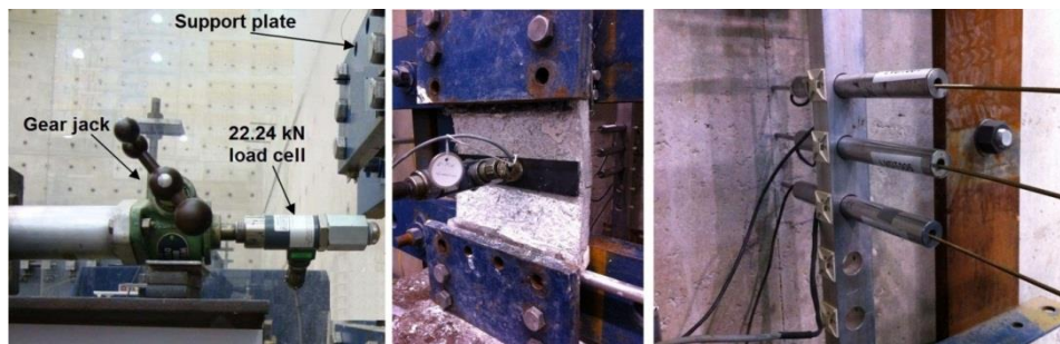
Fig. 3 The static test setup
