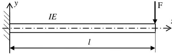
Fig. 1 Clamped-free beam (Cantilever beam)
