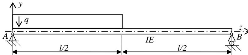
Fig. 2 Simply supported beam
