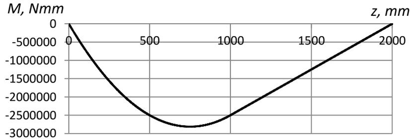
Fig. 3 Moment function of simply supported beam
