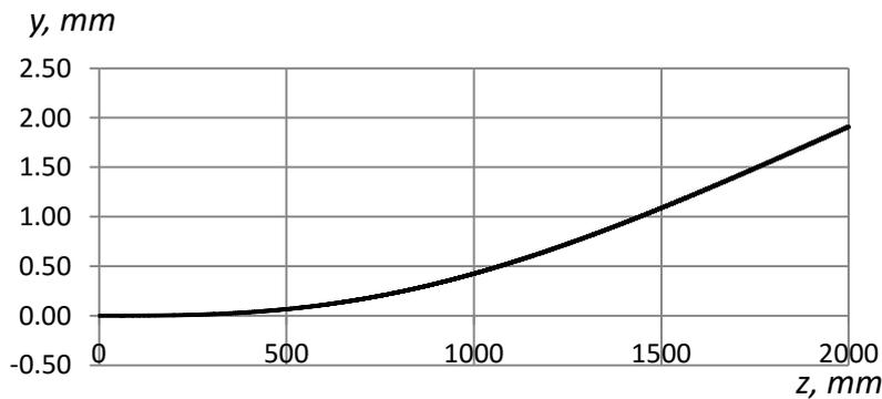
Fig. 4 Elastic curve of the beam for  $y'(0)=0$
