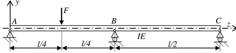
Fig. 6 Beam with three-supports
