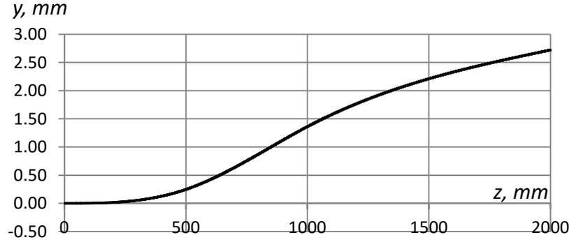
Fig. 8 Elastic curve of the beam in case of  $y'(0)=0$
