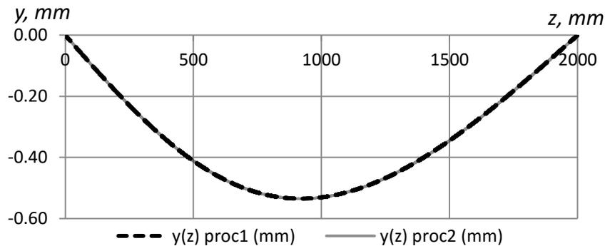
Fig. 5 Elastic curves of the beam obtained by Procedure 1 and 2
