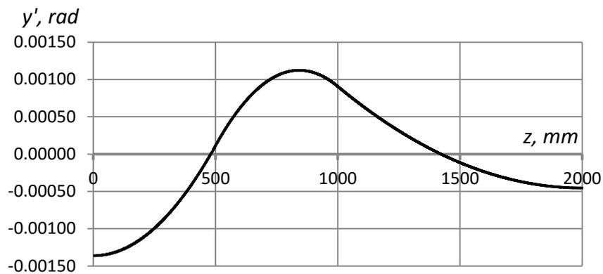
Fig. 10 Slope function of the beam with three supports
