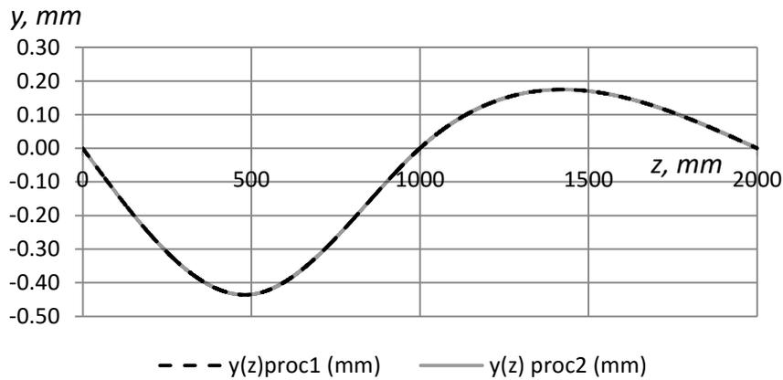
Fig. 9 Elastic curves of the beam with three supports obtained by Procedure 1 and Procedure 2
