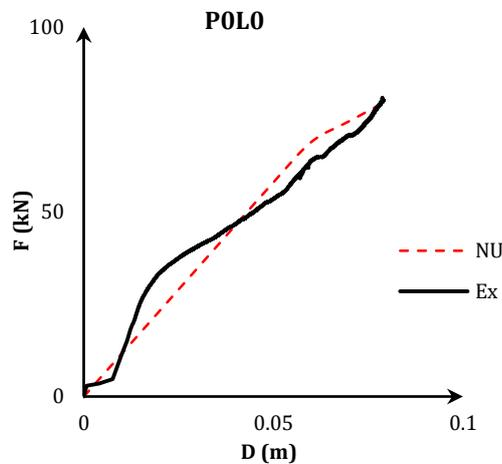
Fig. 6 Force-displacement graphs in numerical and experimental for P0L0
