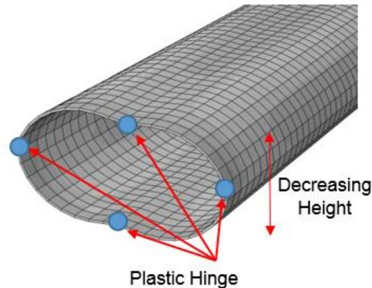
Fig. 7 Failure of non-strengthened specimen (P0L0)
