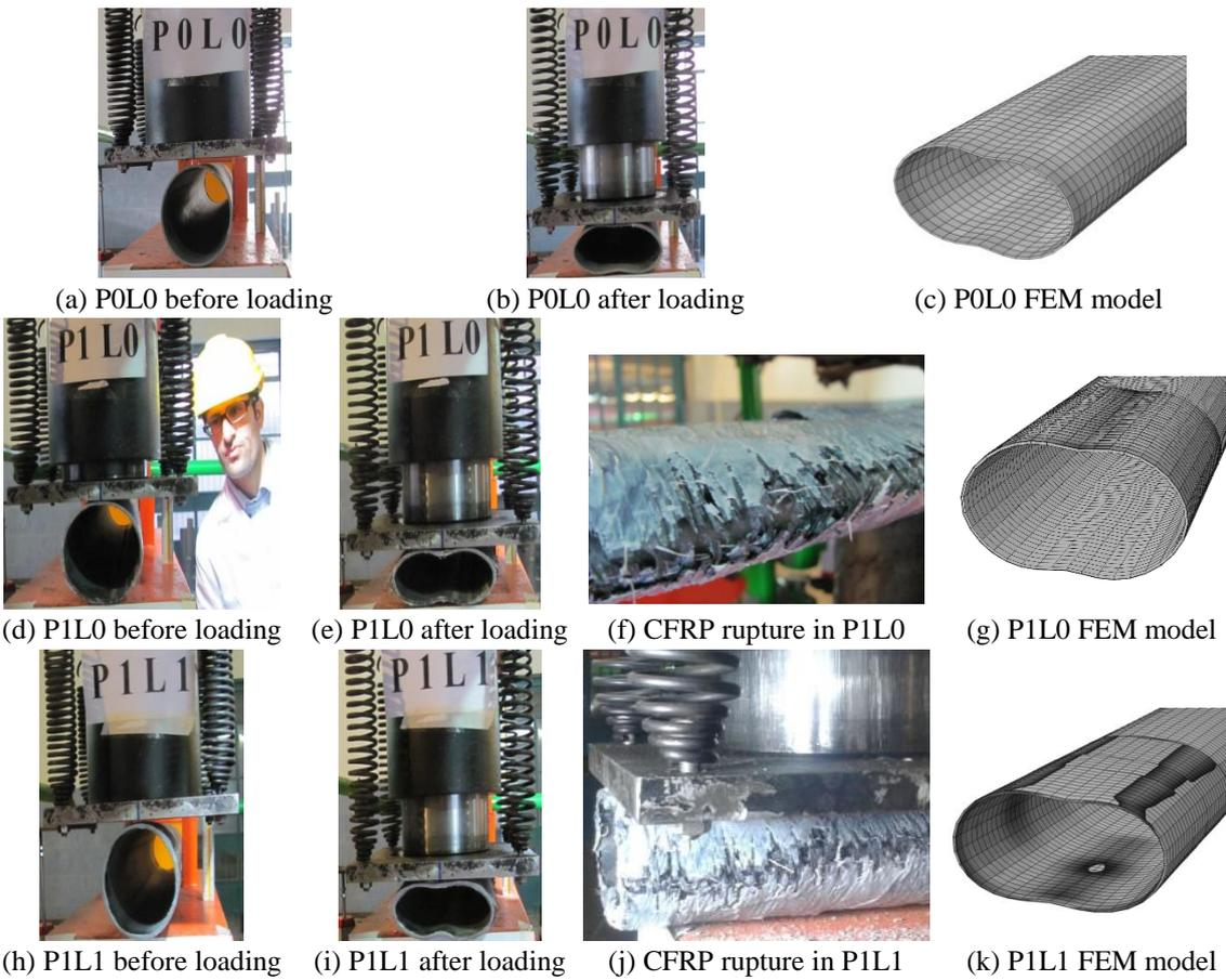
Fig. 4 Experimental and numerical models
