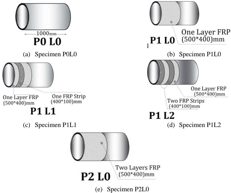
Fig. 1 Schematic of the specimens
