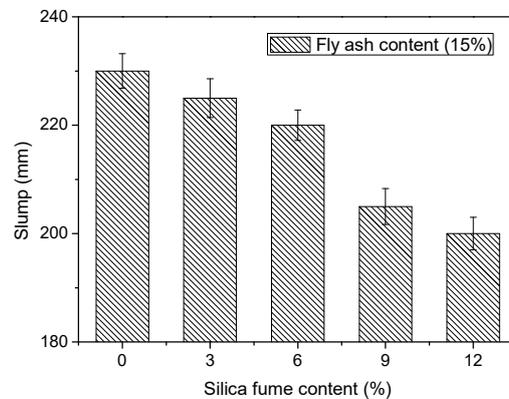
Fig. 6 Effect of silica fume content on slump
