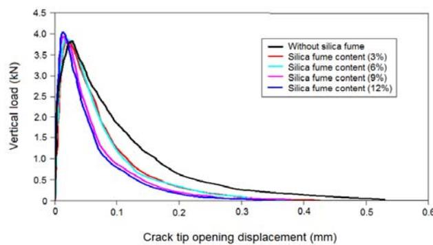
Fig. 14 Contrast of “ $P_v$ - $CTOD$ ” curves of different silica fume content
