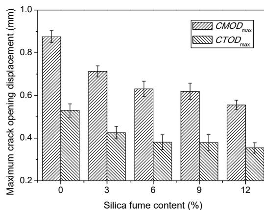
Fig. 16 Effect of silica fume content on maximum crack opening displacement
