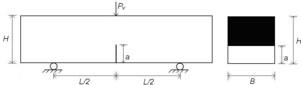
Fig. 1 Shape and size of beam specimen
