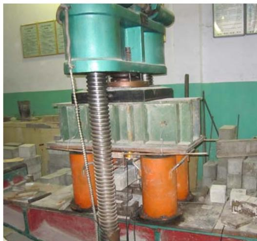
Fig. 3 Loading device of three-point bending test
