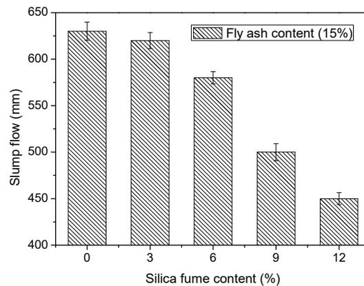
Fig. 7 Effect of silica fume content on slump flow
