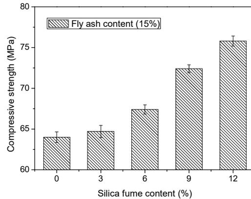
Fig. 8 Effect of silica fume content on compressive strength
