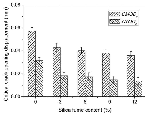
Fig. 15 Effect of silica fume content on critical crack opening displacement
