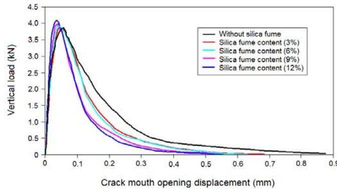
Fig. 13 Contrast of “ $P_v$ - $CMOD$ ” curves of different silica fume content
