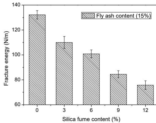
Fig. 11 Effect of silica fume content on fracture energy
