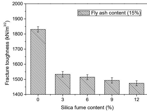
Fig. 10 Effect of silica fume content on fracture toughness
