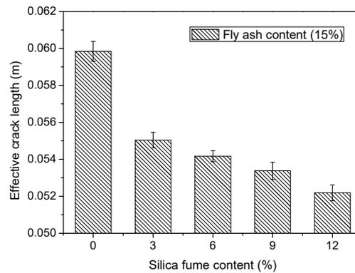
Fig. 9 Effect of silica fume content on effective crack length
