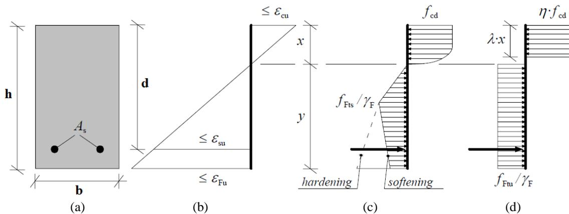
Fig. 20 stress-strain relationship (a) cross section (b) strain distribution (c) actual stress and force distribution (d) simplified stress and force distribution
