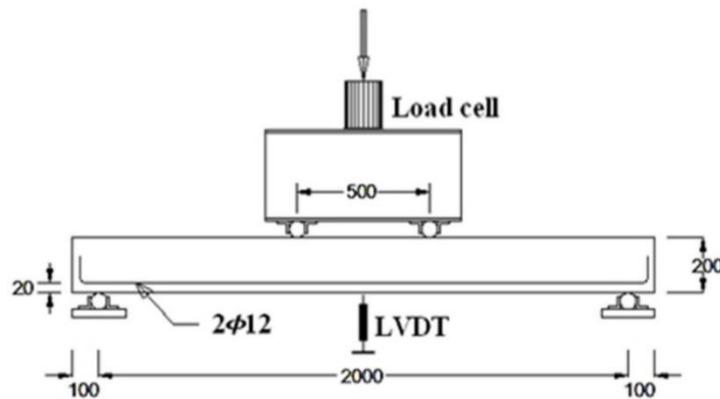
Fig. 5 Test set up
