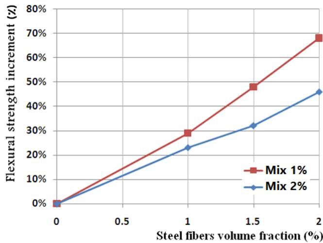
Fig. 19 Flexural strength increment of Mix 1% and Mix 2% beams with different fibers volume fraction
