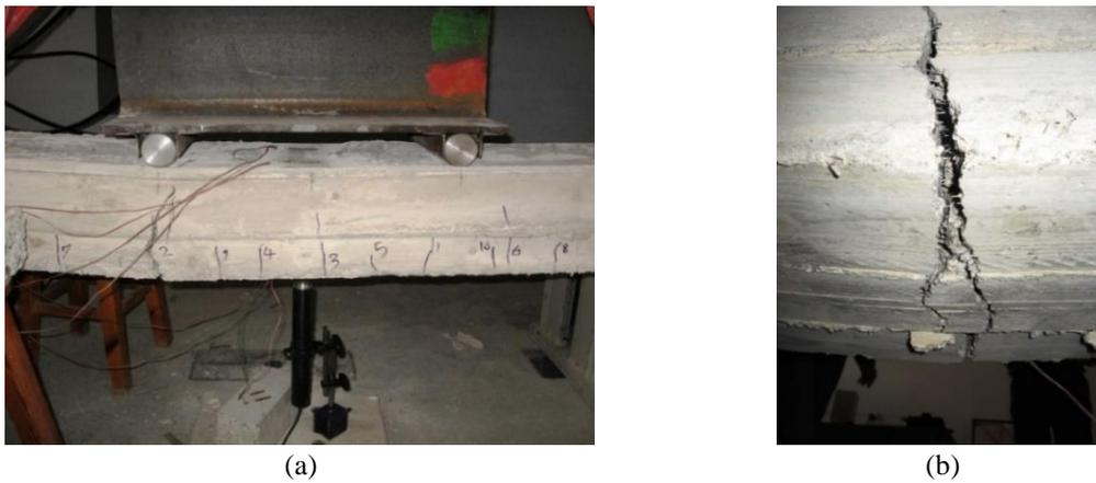
Fig. 15 beam specimen after test (a) general cracks view (b) major flexural crack
