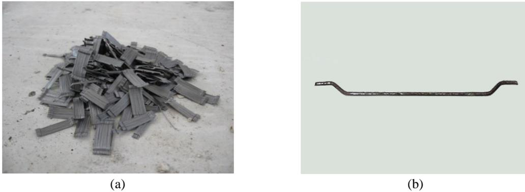
Fig. 1 (a) Steel fibers (b) Single steel fiber (hooked ended)
