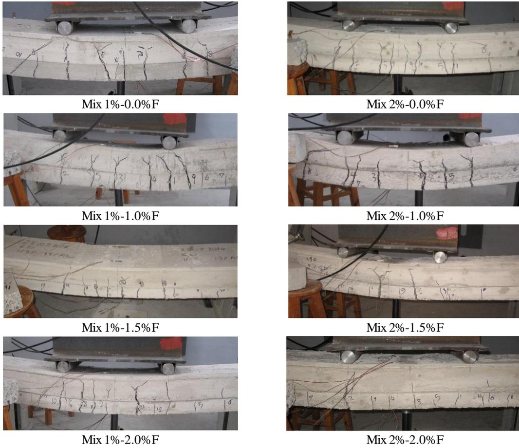
Fig. 22 Failure mode of Mix 1% and Mix 2% beams with different fibers volume fraction
