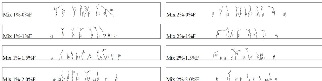
Fig. 21 Cracking pattern of Mix 1% and Mix 2% beams with different fibers volume fraction
