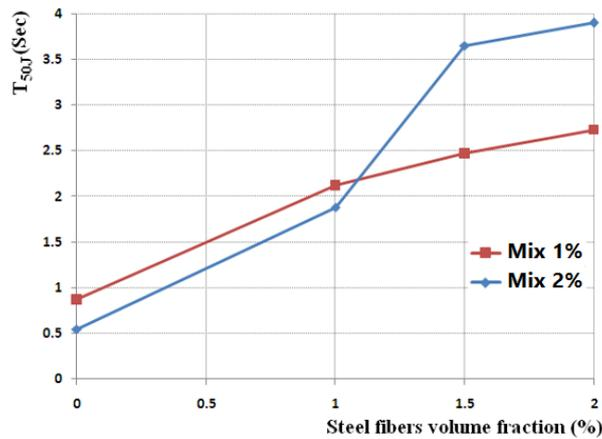
Fig. 11 T<sub>50</sub> time in J-Ring tests
