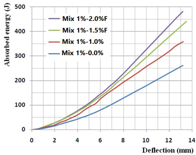
Fig. 23 Absorbed energy vs. deflection curves for Mix 1% beams
