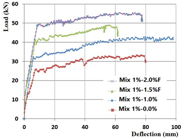
Fig. 16 Load-deflection curves from beams tests performed from Mix 1% with different ratio of steel fibers
