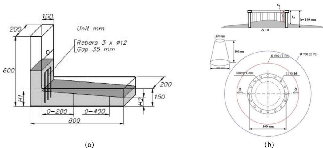
Fig. 4 (a) L-Box test (EFNARC 2005) (b) J ring test (Gencel *et al.* 2011)
