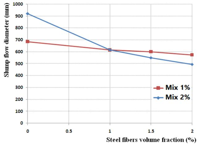
Fig. 8 Slump flow diameter
