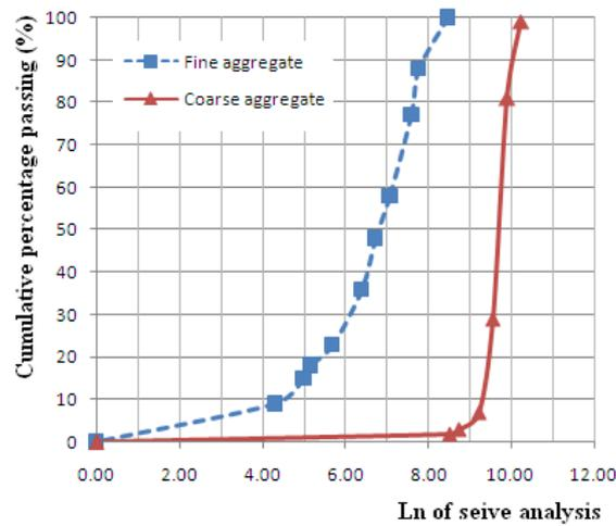
Fig. 2 Sieve analysis grading results
