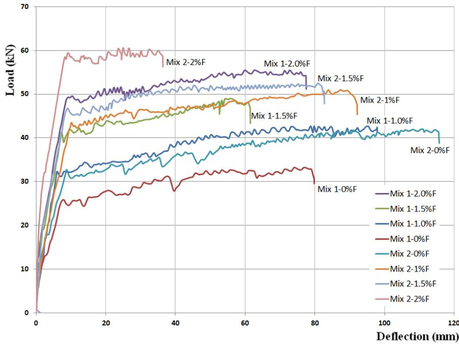
Fig. 18 Load-deflection curves for Mix 1% and Mix 2% beams with different ratio of fibers
