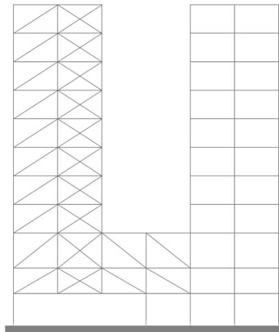
Fig. 11 modeling of the equivalent compression struts (DC2)
