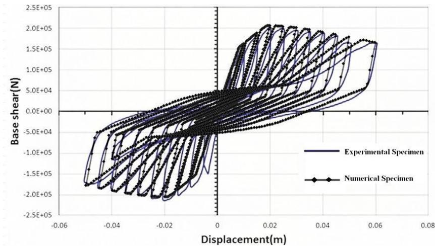
(c) Load-displacement relation for the specimen
