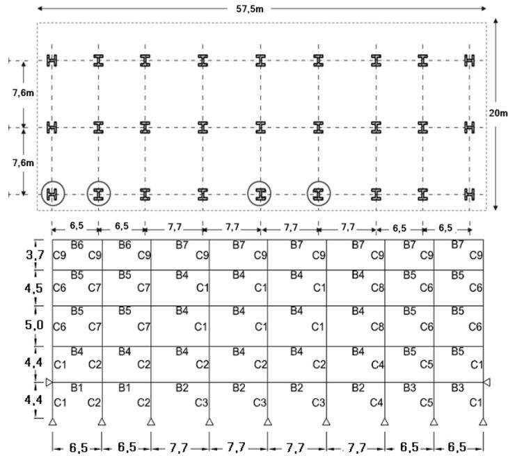
(c) Columns and beams plan and location of removal columns
