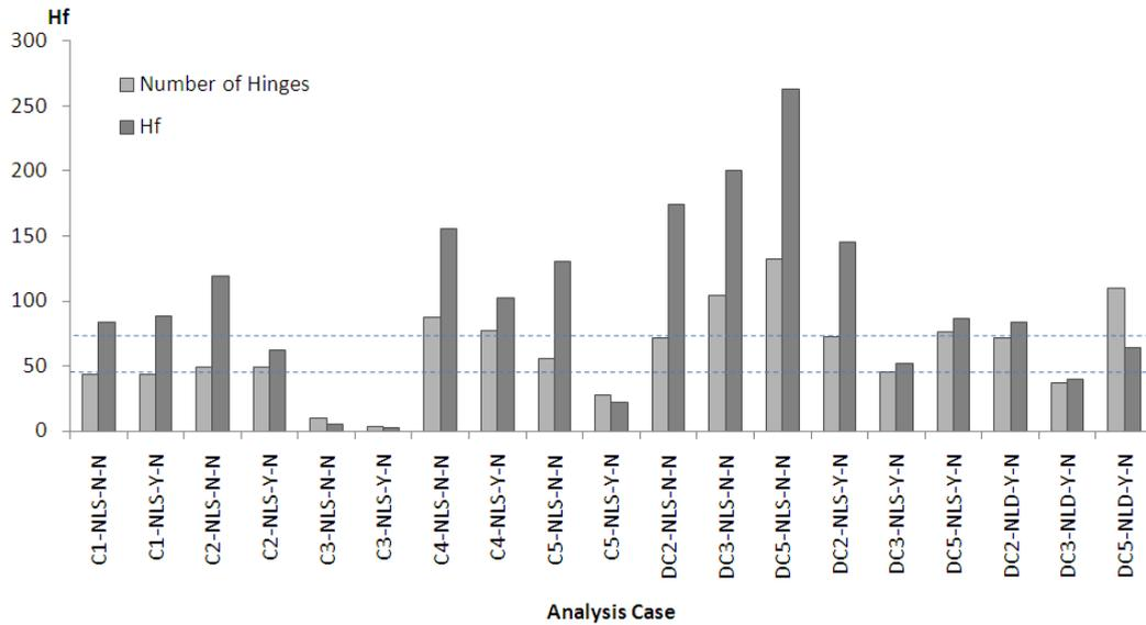
Fig. 17 hazard factor ( $H_f$ ) for different analysis case
