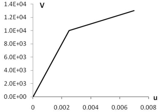
(b) monotonic lateral force-deformation bilinear curve for URM infill panels
