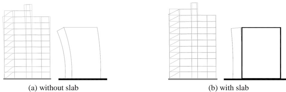
Fig. 12 deformed shape of the structure in C1-NLS method (scale factor: 15)
