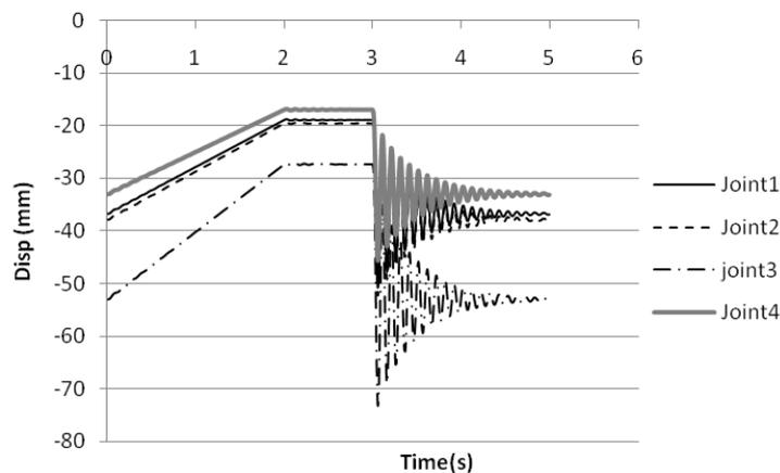
Fig. 5 Time-history of displacement of the four removed columns top joints
