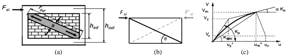
Fig. 2 (a) equivalent compression-concentric strut model, (b) modeling of strut based on lateral load direction, (c) strength envelope for masonry infill panels based on constitutive model for masonry
