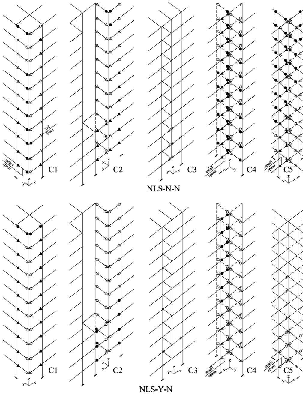
Fig. 14 hinges formation in single column removal scenarios
