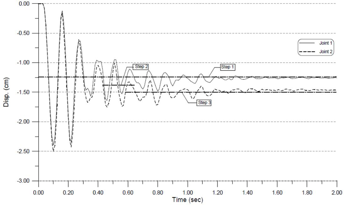
Fig. 16 time-history diagrams of  $d_s$  in NLD-Y-Y-DC2 scenario
