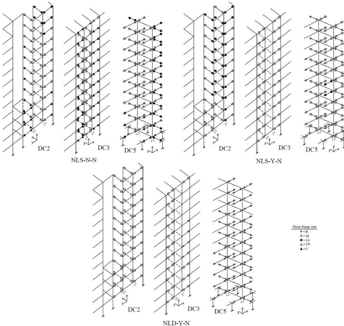
Fig. 15 hinges formation in double columns removal scenarios
