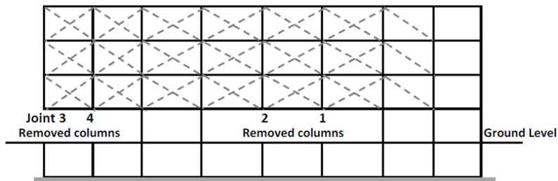
(d) Location of removal columns and equivalent struts in elevation view
