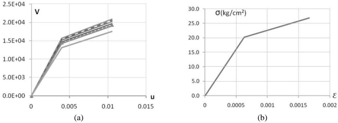
Fig. 10 (a) monotonic lateral force-deformation bilinear curve for URM infill panels, (b) normalized stress-strain curve
