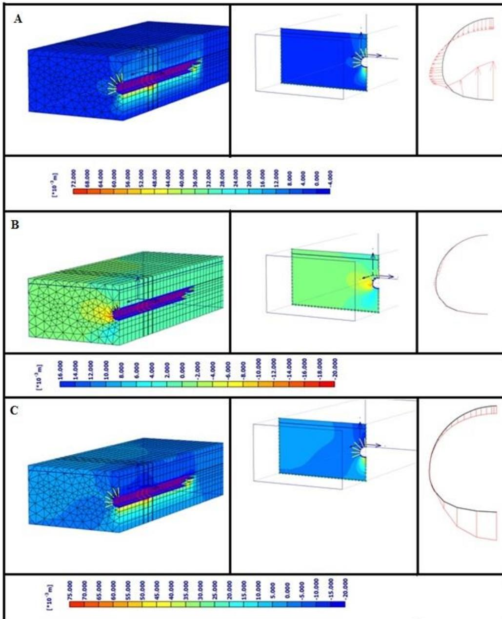
Fig. 12 Results of the time dependent numerical analysis for NDSS ((A) Total deformation (in mm), (B) Axial deformation in (mm), (C) Vertical deformation (in mm))
