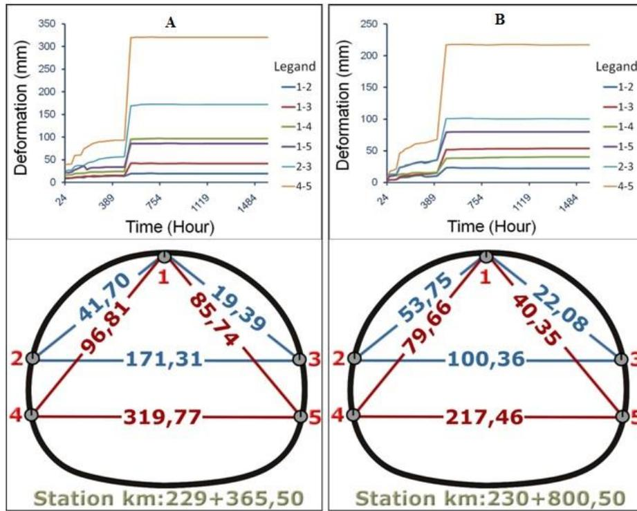
Fig. 7 Tape ekstensometer deformation measurements to determine horizontal and vertical closure of tunnel sections ((A) KM:229+365.50; (B) KM:230+800.50)
