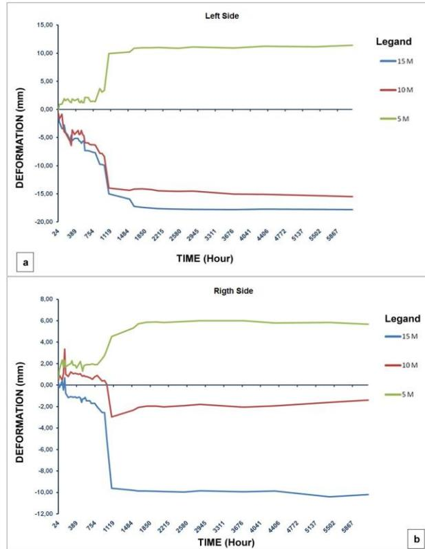
Fig. 10 The graph of rod-extensometer measurements taken from KM: 229+400.20 ((a) Left Side rod-extensometer, (b) Right Side rod-extensometer)
