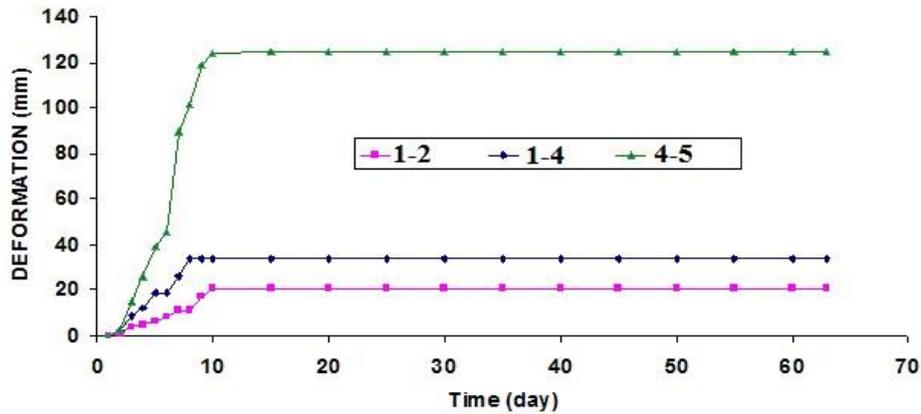
Fig. 13 Predicted convergence amount on the measurement points on Tunnel 34
