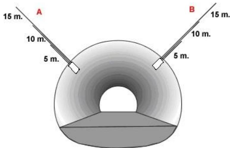
Fig. 9 The schematic views of the rod-extensometer application at Tunnel 34
