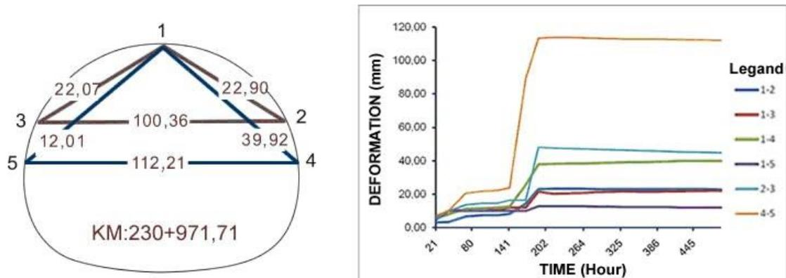
Fig. 14 Results of the tape extensometer measurements after NDSS application at KM: 230+971.71 (Left side-Cross-section of tunnel, Right side-Time-dependent measurements between points)
