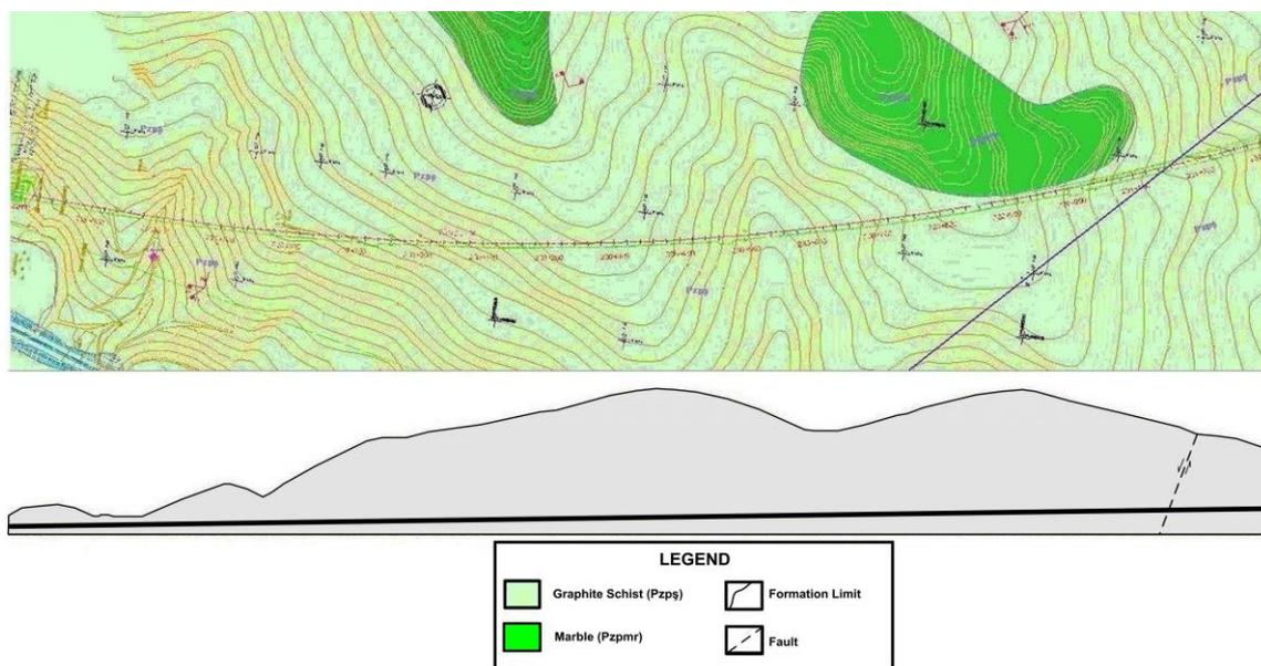
Fig. 4 The geological map and geological cross-section of Tunnel 34 (re-design from Şimşek *et al.* 2009)
