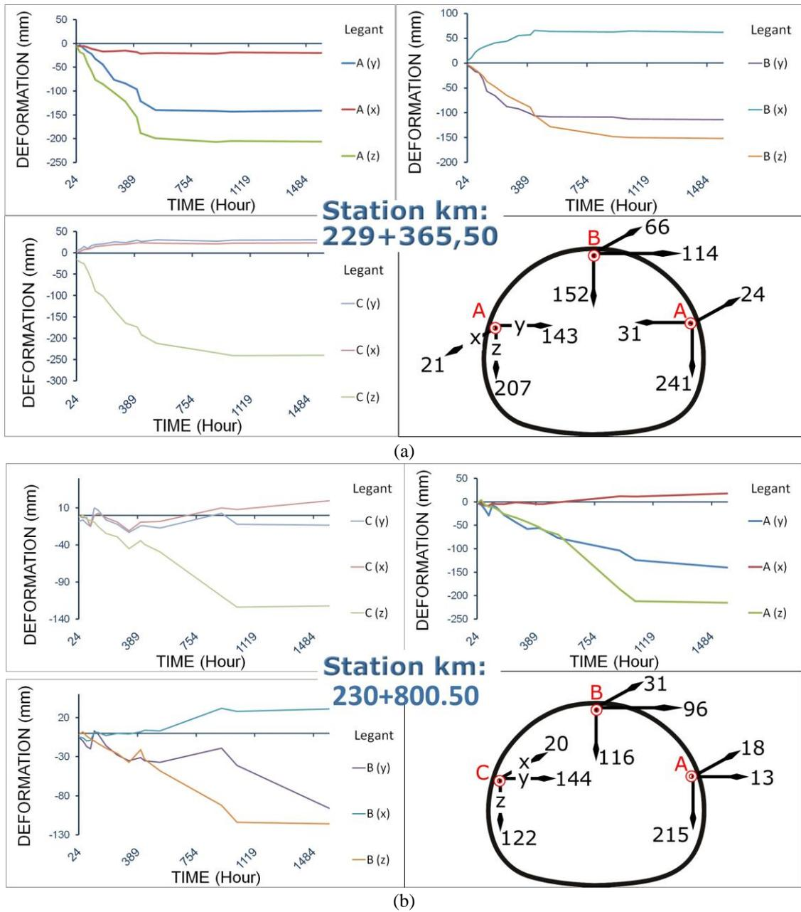
Fig. 6 Opto-trigonometric deformation measurements ((a) KM:229+365.50, (b) KM:230+800.50)
