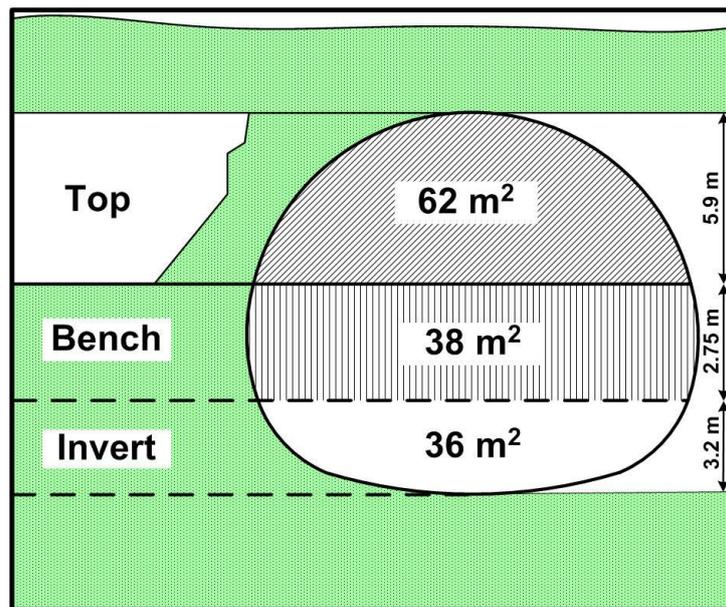
Fig. 5 Excavation geometry of Tunnel 34 (Şimşek *et al.* 2009)
