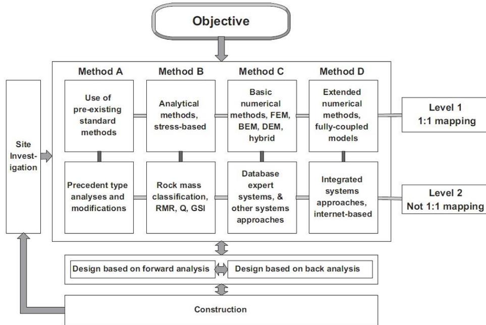
Fig. 1 Flowchart of rock mechanics modeling types used to support rock engineering design (Feng and Hudson 2008)
