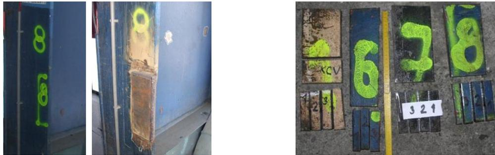
(a) A column before and after the collection of specimens with a treatment of the flange after sampling (b) A separation of elements for a generation of specimens for tensile tests
