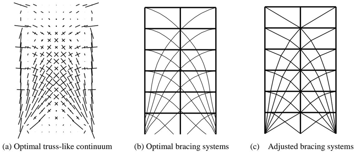
Fig. 3 Optimal structure of example 1
