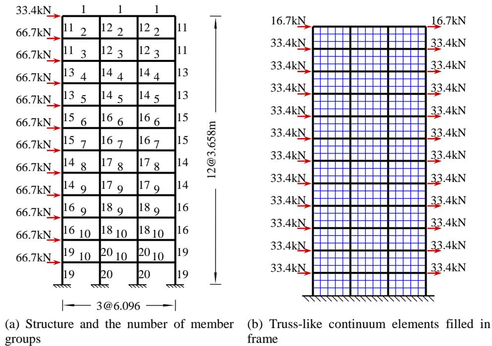
Fig. 5 Mechanics model of example 2
