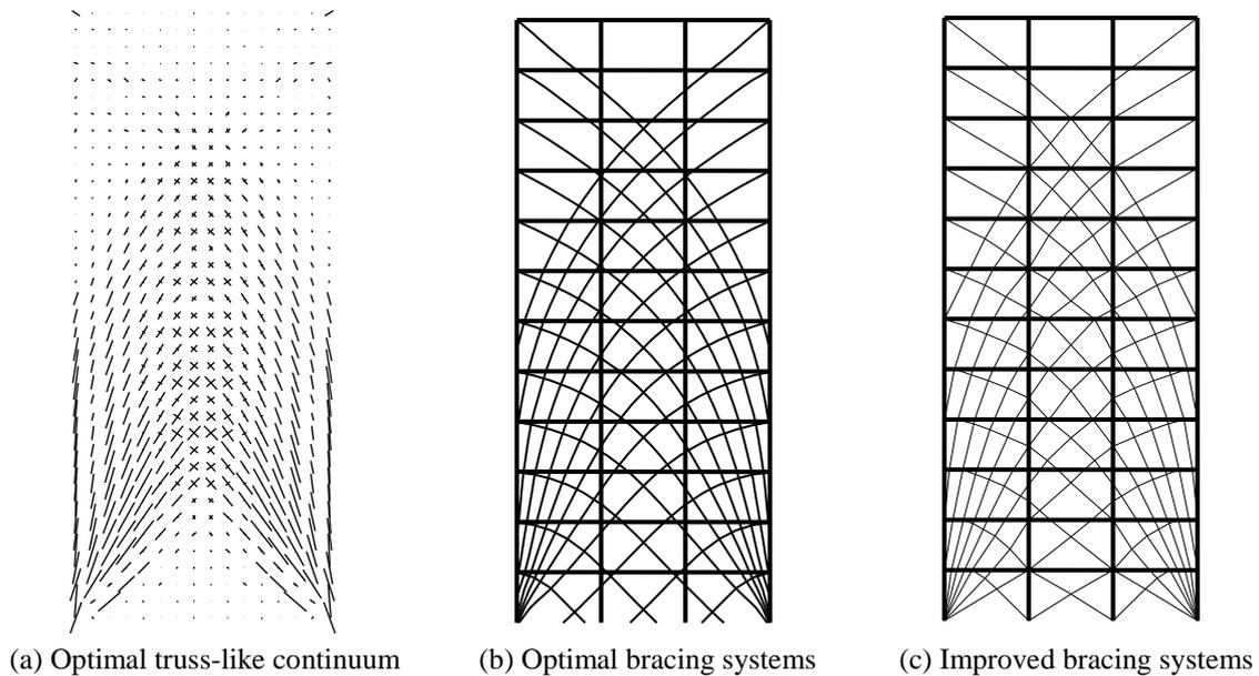
Fig. 7 Optimal bracing structure of example 2
