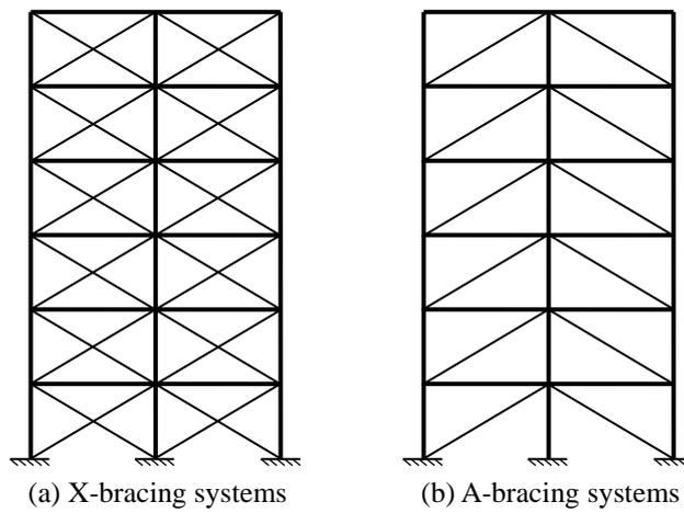
Fig. 4 Frame with bracing systems of example 1
