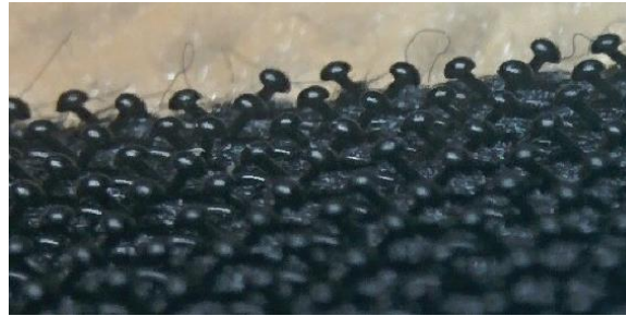
Fig. 2 Mushroom-shaped head hook of improved Velcro
