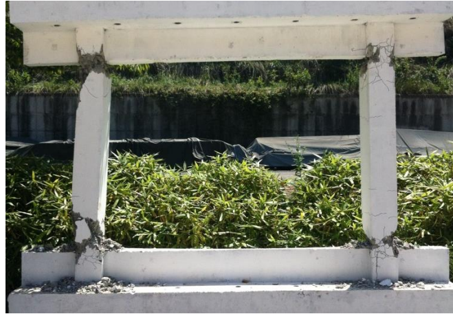
(c) Collapsed plastic hinge zone at column
