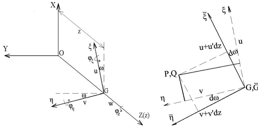
Fig. 1 Global and local coordinate of pre-twisted thin-walled beam
