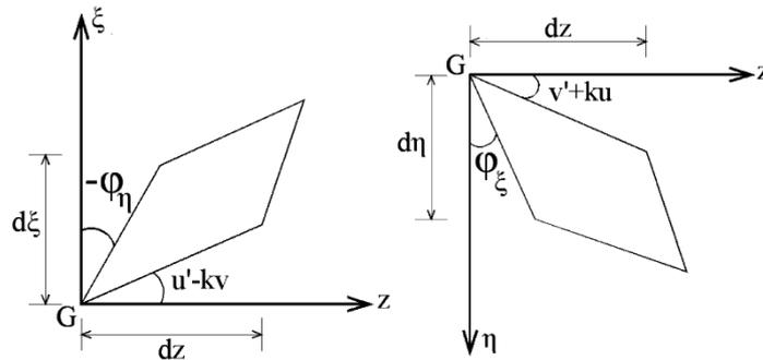
Fig. 2 Infinitesimal element shear strains of pre-twisted thin-walled beam
