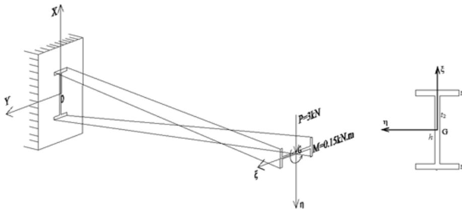
Fig. 6 the geometric parameter of pre-twisted beam with I cross section
