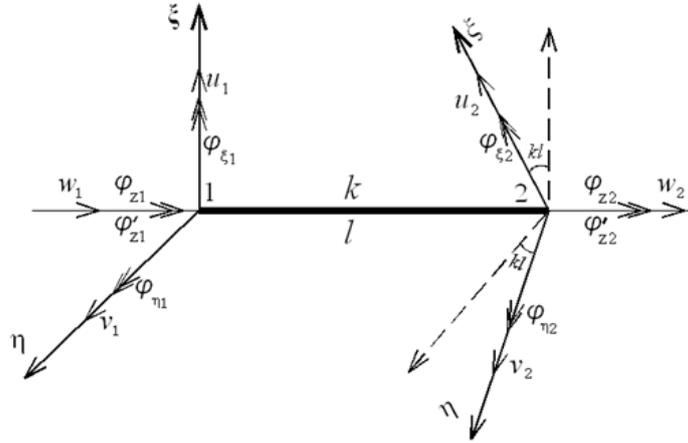
Fig. 3 The node displacement of pre-twisted thin-walled beam
