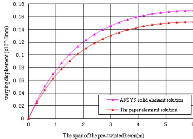
Fig. 7 The pre-twisted beam warping displacement comparison with  $I$  cross section
