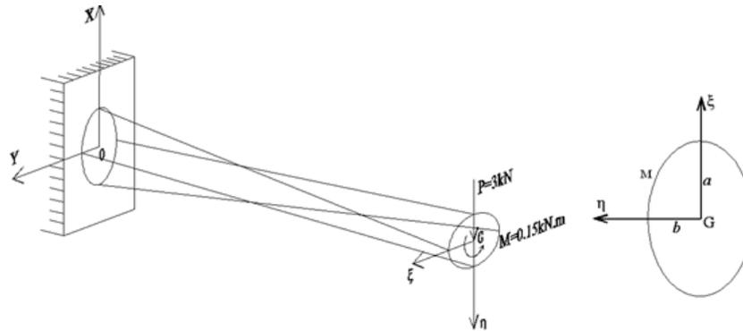
Fig. 4 the geometric parameter of pre-twisted ellipse beam ( $a=200$  mm,  $b=100$  mm)
